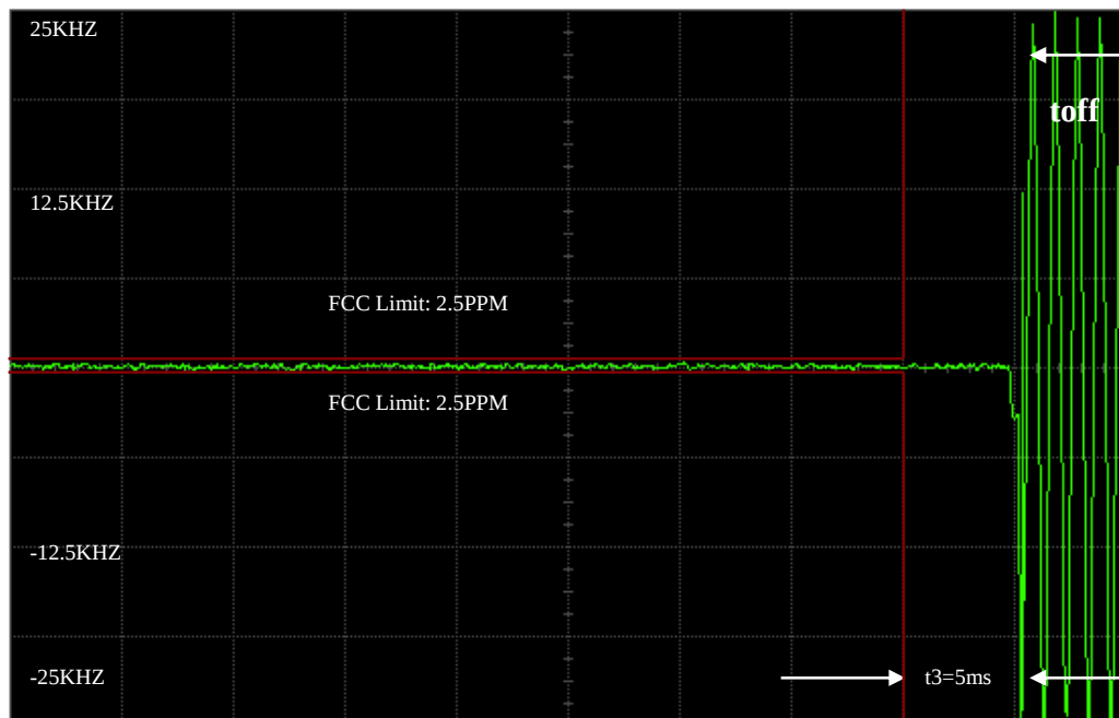
Figure 6I-4: 5.5 Watts, 25 kHz, 143.025 MHz, De-Key Decay Time
