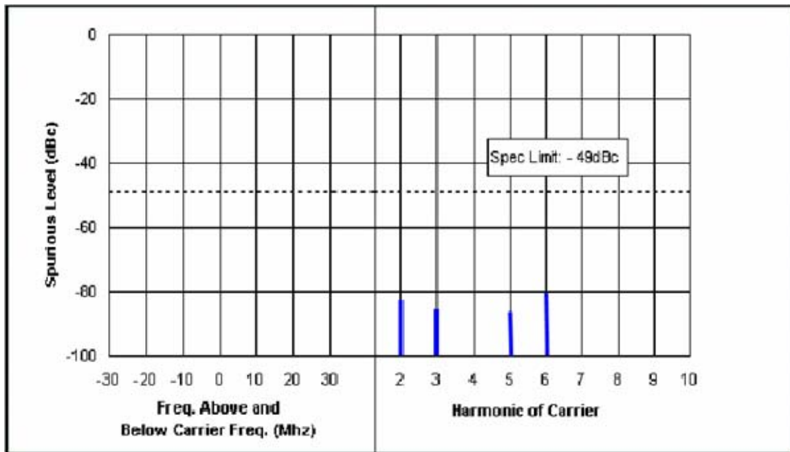
6G-1: Hi-Power Harmonic of Carrier 450.025 MHz, 25 kHz Channel Spacing
