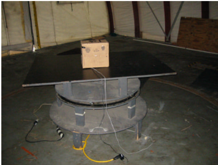
Transmitter Spurious Test Setup, Back View
