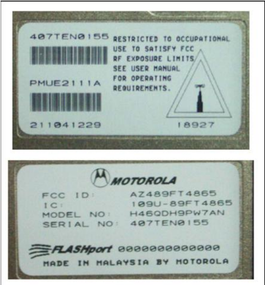
Figure 3-11: Close-up view of FCC & RF Safety Label
