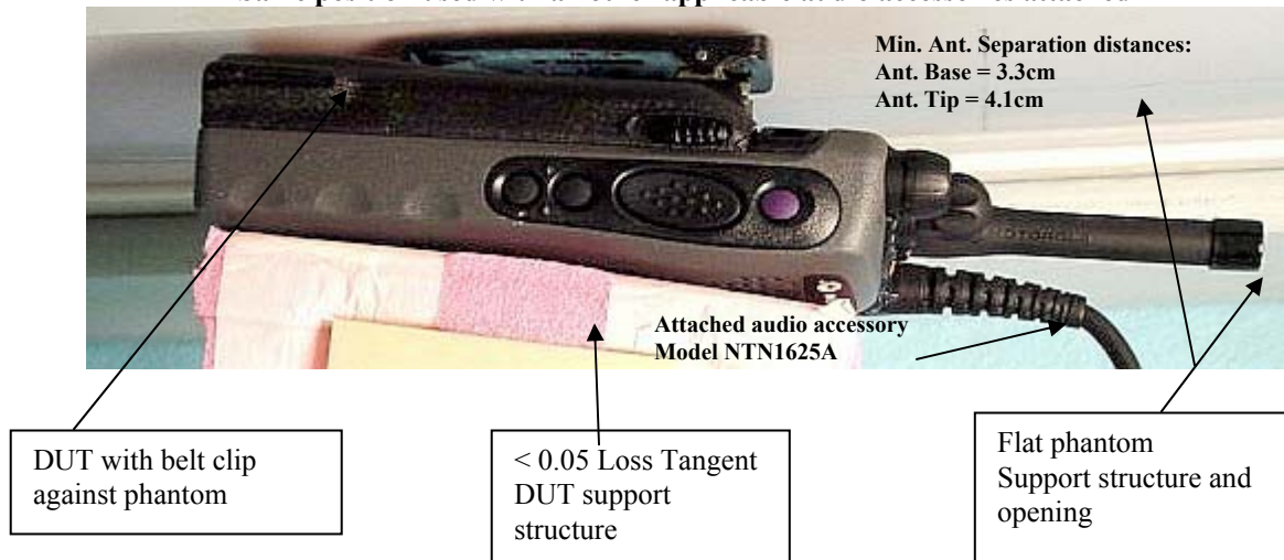
Figure 2. Assessment @ the body w/ antenna model NAE6546AR. DUT with belt clip accessory model HLN9844A against the phantom, with attached audio accessory NMN6191C
