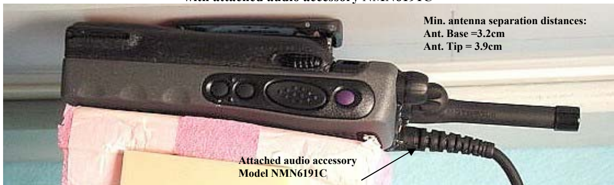
Figure 2. Assessment @ the body w/ antenna model NAE6546AR. DUT with belt clip accessory model HLN9844A against the phantom, with attached audio accessory NMN6191C
