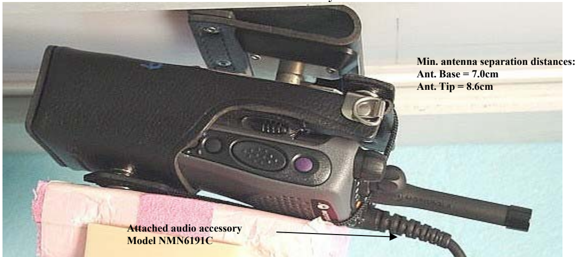
Figure 4. Assessment @ the body w/ antenna model NAE6546AR. DUT with carry case accessory model NNTN4116A against the phantom with attached audio accessory model NMN6191C
