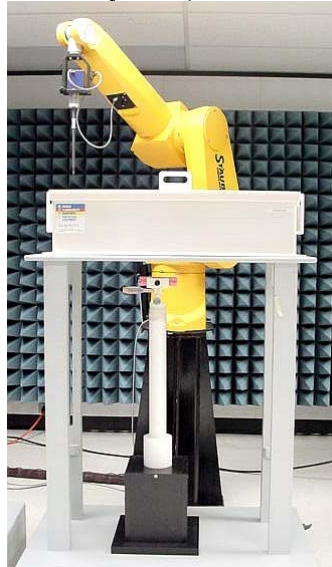
Figure 10: Robot Test System (Flat Phantom used for face)
