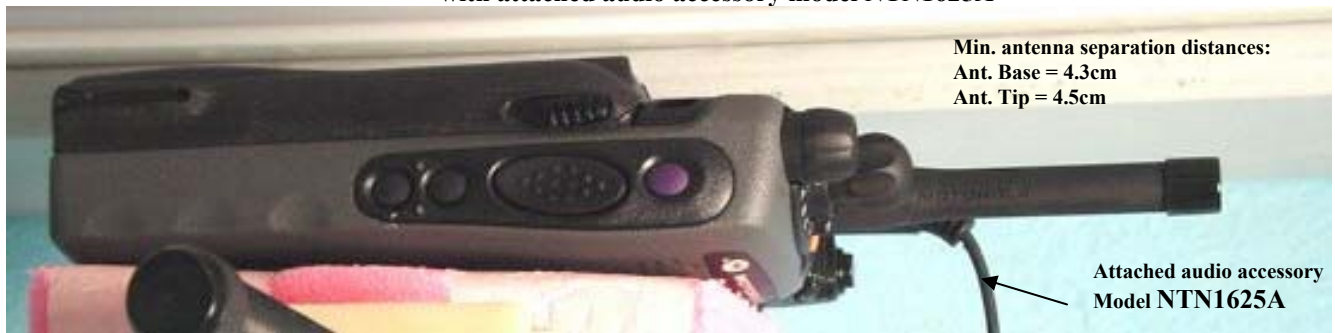
Figure 7. Assessment @ the body with antenna NAE6546AR. DUT with back separated 2.5cm from the phantom with attached audio accessory model NTN1625A
