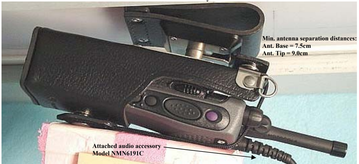
Figure 5. Assessment @ the body w/ antenna model NAE6546AR. DUT with carry case accessory model NNTN4117A against the phantom with attached audio accessory model NMN6191C
