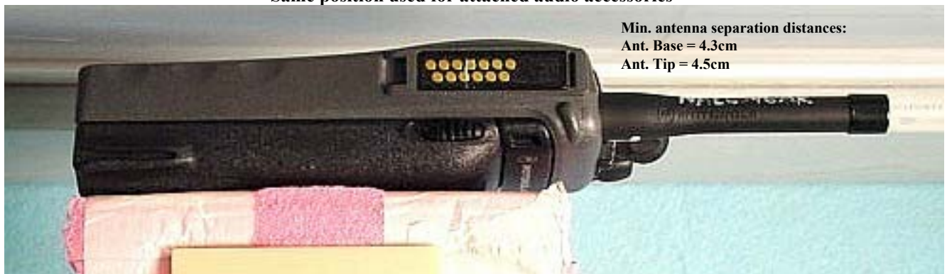
Figure 8. Assessment @ the face w/ antenna model NAE6546AR. DUT with front housing separated 2.5cm from the phantom Same position used for attached audio accessories
