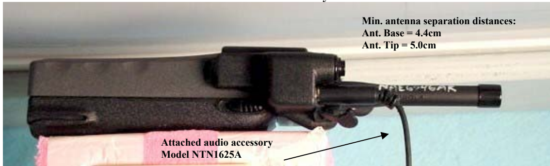
Figure 6. Assessment @ the body with antenna NAE6546AR. DUT with front separated 2.5cm from the phantom with attached audio accessory model NTN1625A
