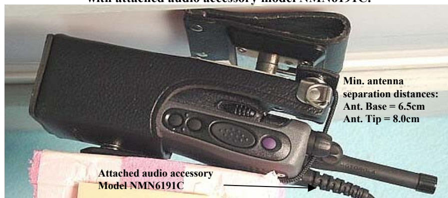
Figure 3. Assessment @ body w/ antenna model NAE6546AR. DUT with carry case accessory model NNTN4115A against the phantom with attached audio accessory model NMN6191C.
