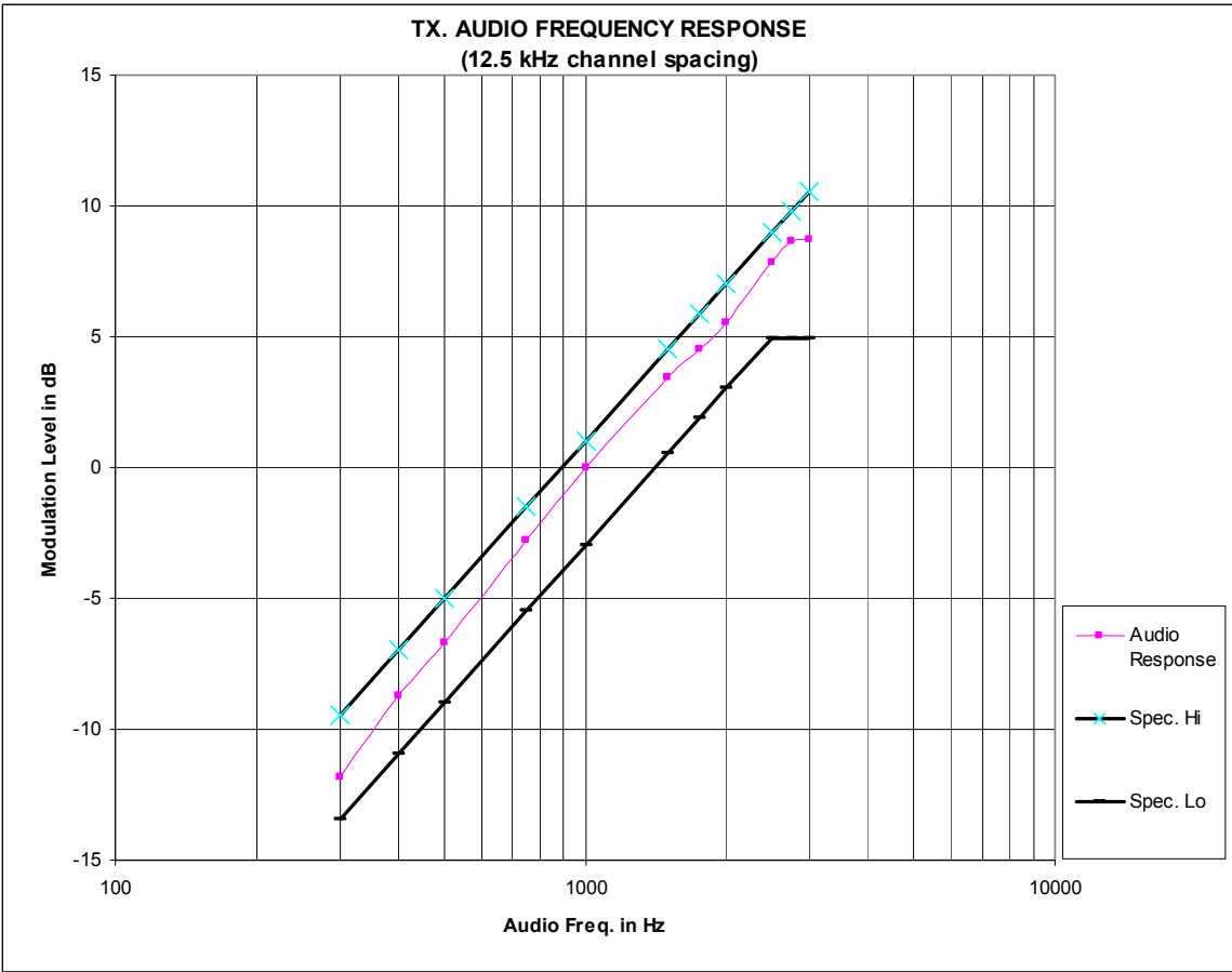
Figure 6B-1: 12.5 kHz Channel Spacing, 425.0125 MHz, Transmit Audio Frequency Response
