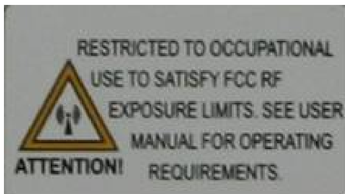
Figure 3-7: Close-up view of RF Safety Label
