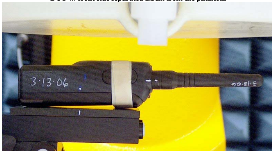
Figure 2: Highest SAR Test Position (face) DUT w/ front side separated 2.5cm from the phantom
