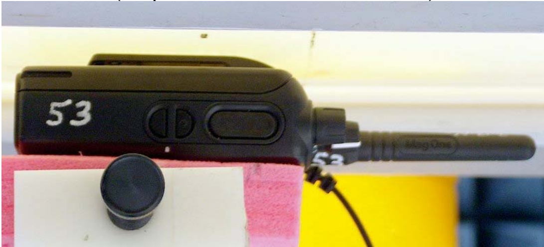
Figure 1: Highest SAR Test Position (Body) DUT w/ belt clip PMLN4691A against the phantom; worst case audio accessory PMLN4658A attached (same position used for all other audio/data accessories)
