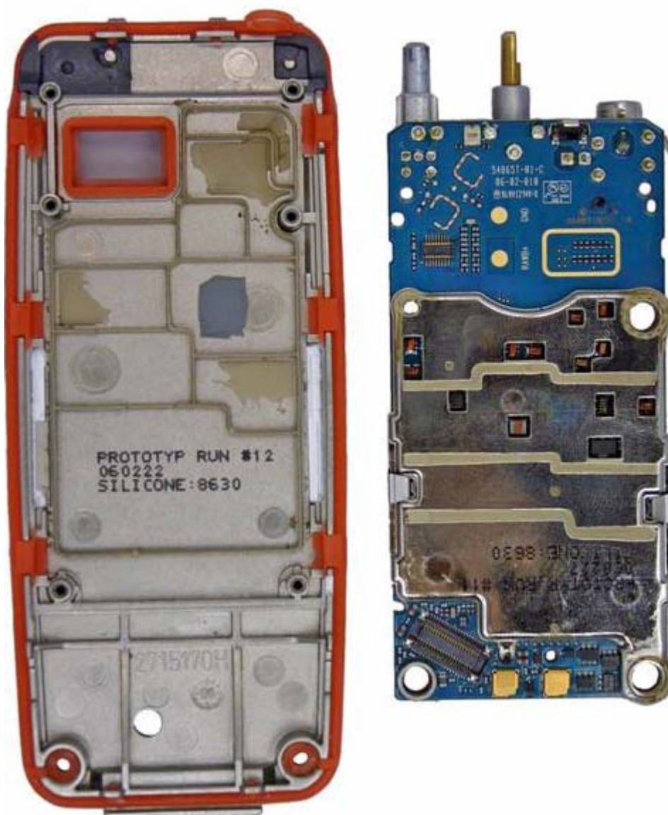
FIGURE 3-4: MOTOTRBO CHASIS, BOARD AND CLIP – SHIELD.
