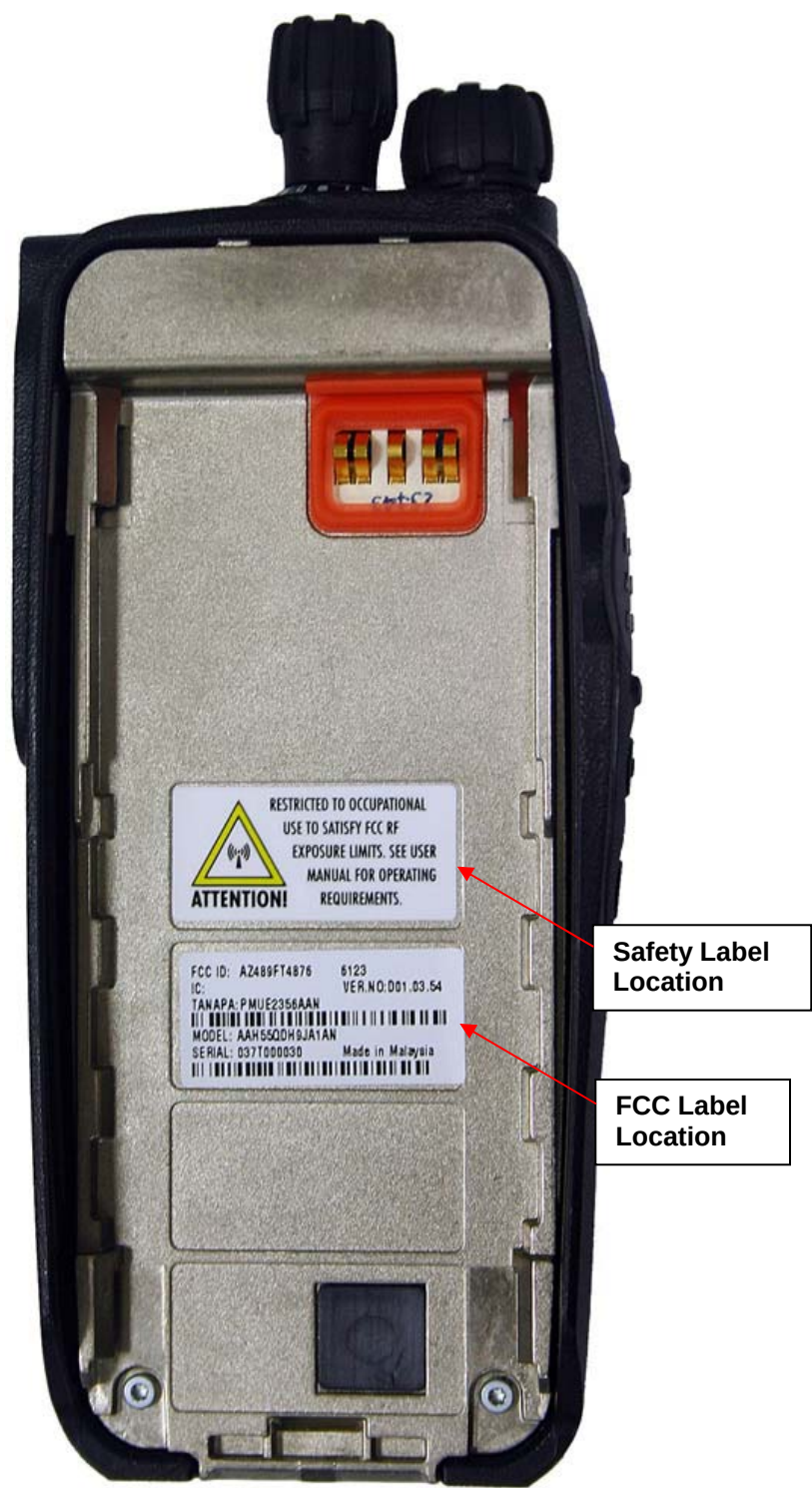
FIGURE 3-6: FCC AND SAFETY LABELS LOCATION OF MOTOTRBO
