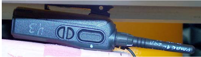
Figure 4: Body Assessment DUT w/ belt clip PMLN4741A against the phantom. With audio acc. Model PMMN4013A attached
