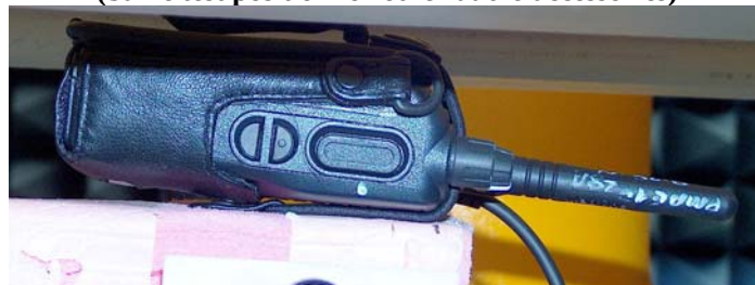
Figure 3: Body Assessment DUT w/ belt clip PMLN4743A against the phantom. Worst case audio acc. Model PMLN4444A attached (Same test position for other audio accessories)
