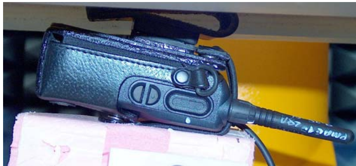
Figure 5: Body Assessment DUT w/ belt clip PMLN4742A against the phantom. With audio acc. Model PMMN4013A attached
