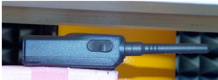
Figure 2: Highest S.A.R. Test Position (face) DUT w/ front side separated 2.5cm from the phantom No audio cable attached
