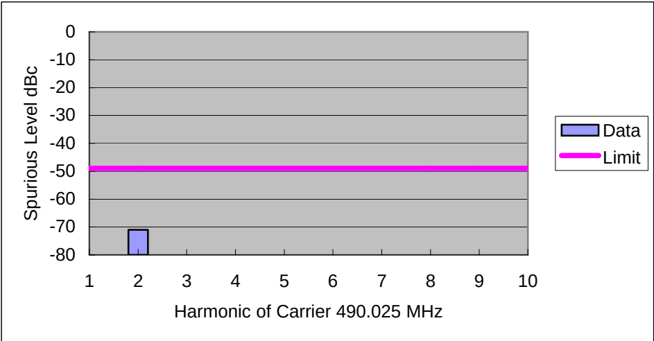
Figure 6F-10: 4.5 Watt Harmonic of Carrier 490.025 MHz, 25 kHz Channel Spacing
