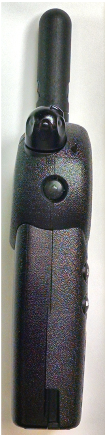
Figure 3-7 Side View Power/Volume Knob & Call Button
