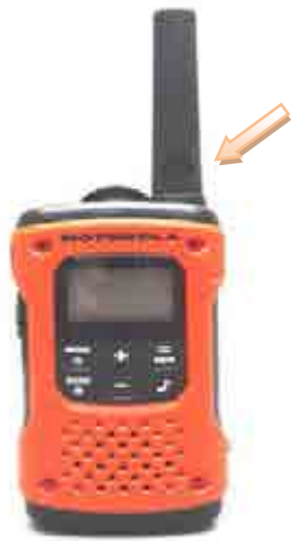
Fixed antenna pointed with arrow (Antenna model: EAN.144F.823RA1)
