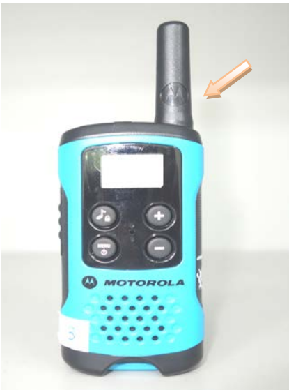
Fixed antenna pointed with arrow
