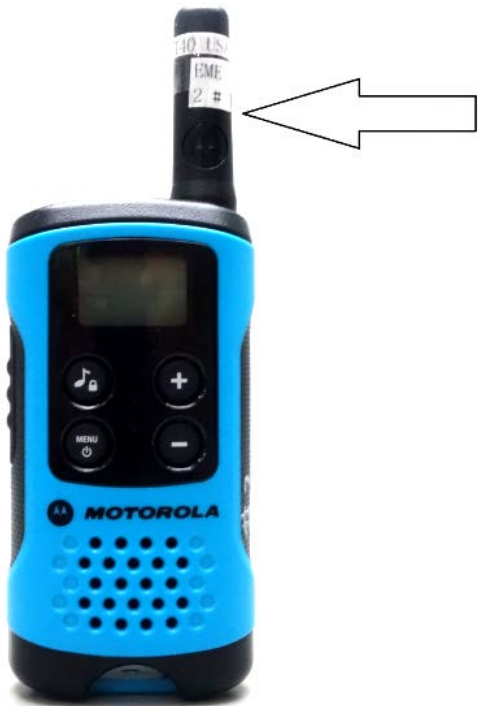
Fixed antenna pointed with arrow
