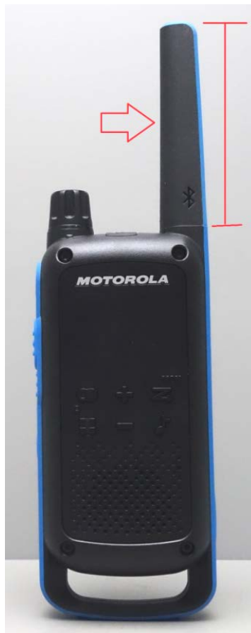
Fixed antenna pointed with arrow (Antenna model: 328010048)
