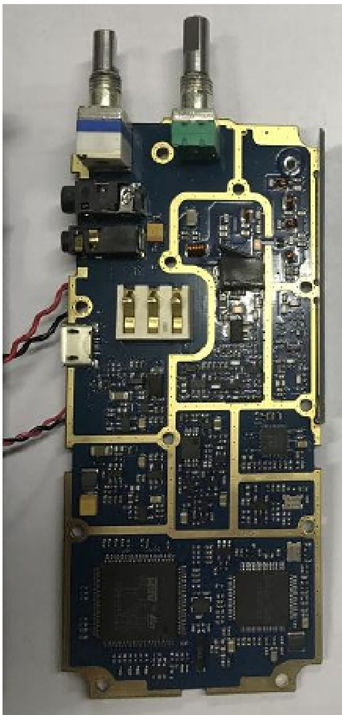
RF board without Shields (Bottom) (BC250D)
