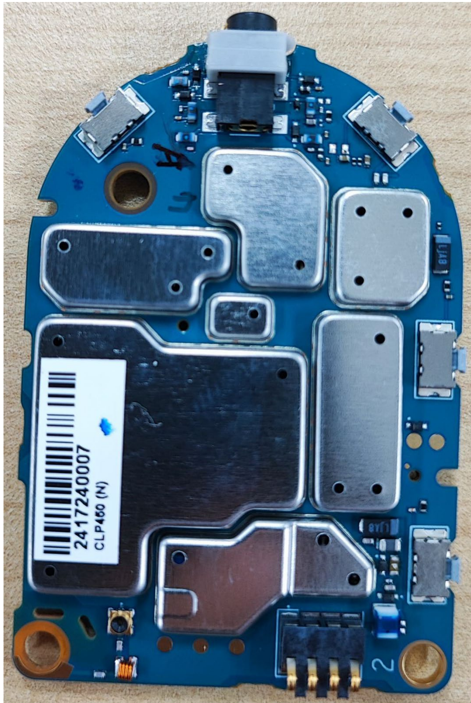
RF board with Shields (Bottom) (CLP1080e, CLP1083e, CLP1010e, CLP1013e)
