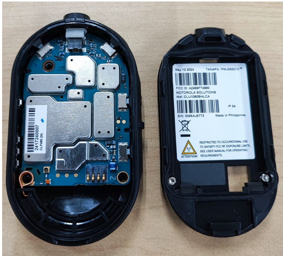
Chassis and Housing (Back side) (CLP1080e, CLP1083e, CLP1010e, CLP1013e)
