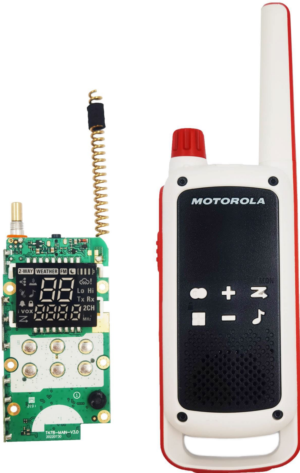
EXHIBIT 9E - RF boards with chassis and housing for (Front Side)
