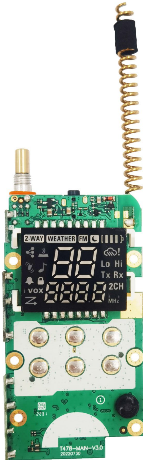
EXHIBIT 9A - RF board with Shields (Top)
