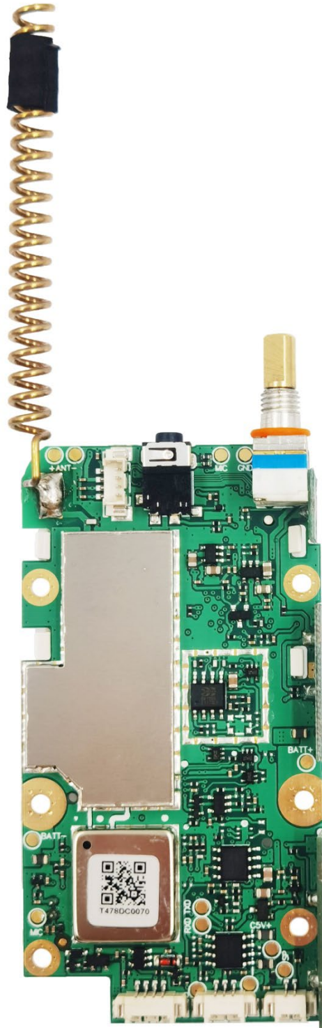
EXHIBIT 9C - RF board with Shields (Bottom)
