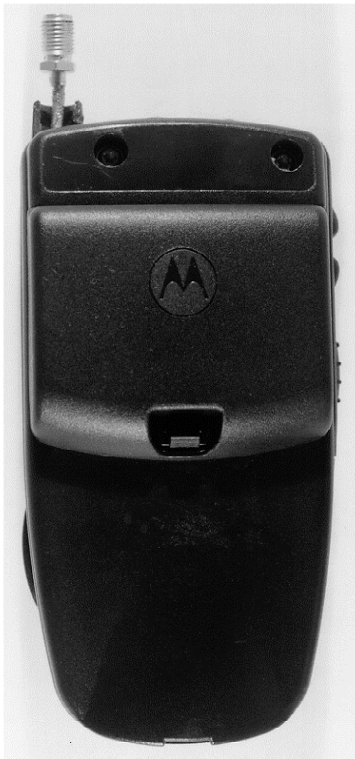
Photograph 7-4: Back view of radio with battery, with a semi rigid cable with female SMA connector soldered on the main circuit board, and enclosed in modified housing for RX/TX conducted emission testing.
