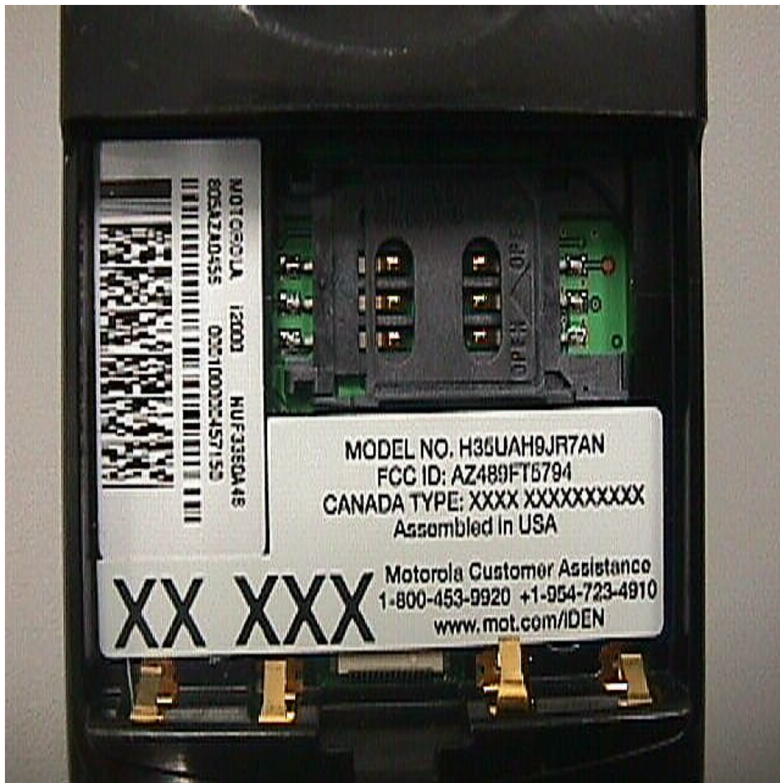
Photograph 3-3: Rear view of radio, showing FCC label
