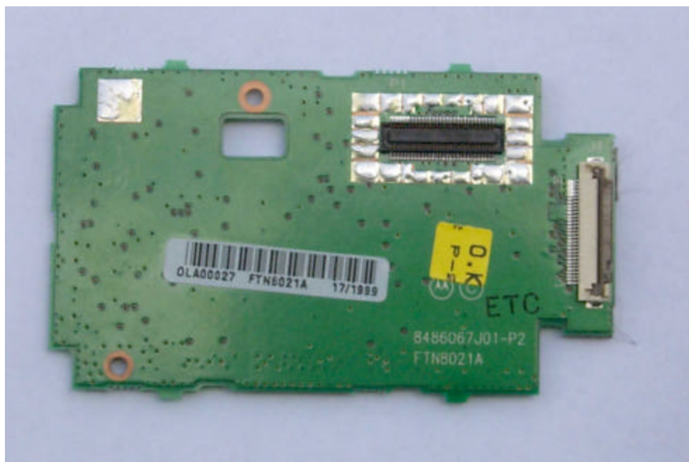
Photograph 9-3: Top side of transceiver Logic Board.
