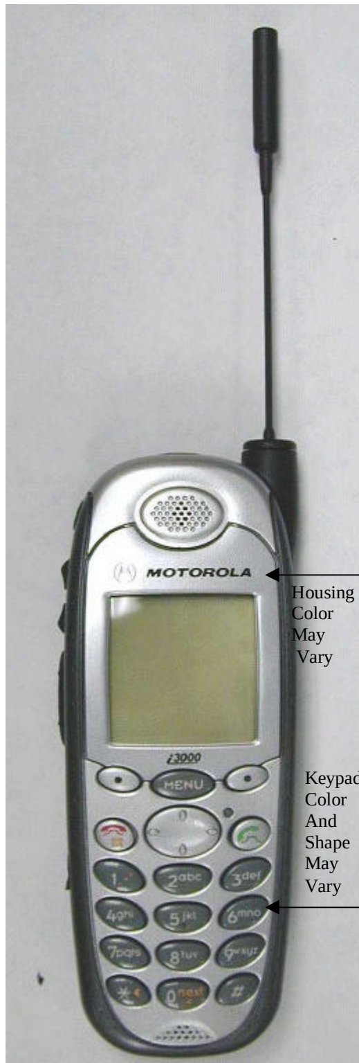
Photograph 3-2: Front View of radio, antenna extended.
