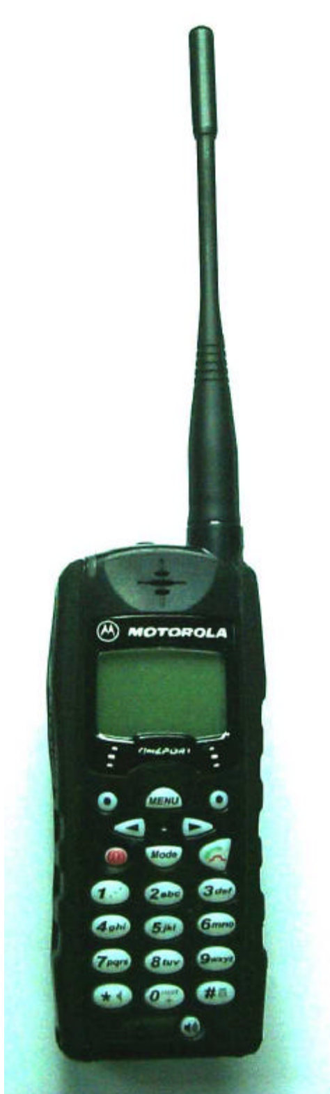
Photograph 3-1: Front view of the radio with \ell/2 top load antenna
