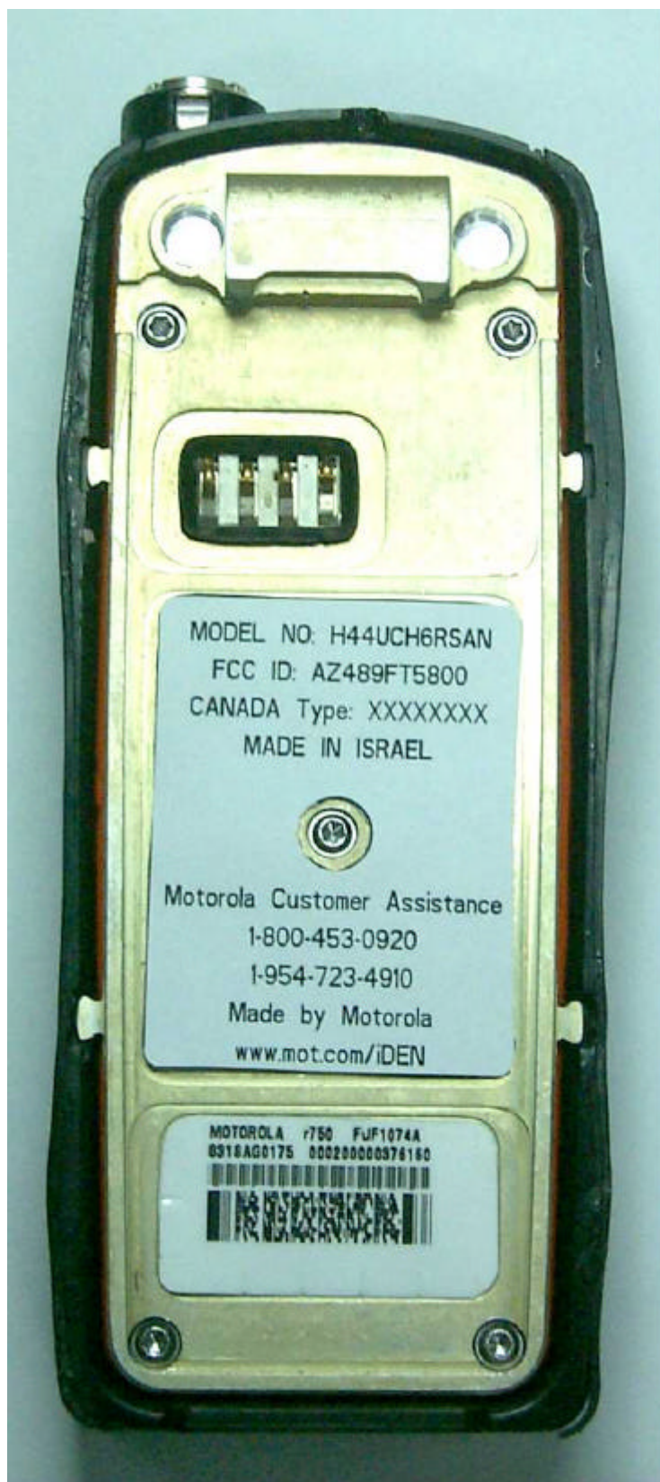
Photograph 3-3: Rear view of the radio, showing FCC label
