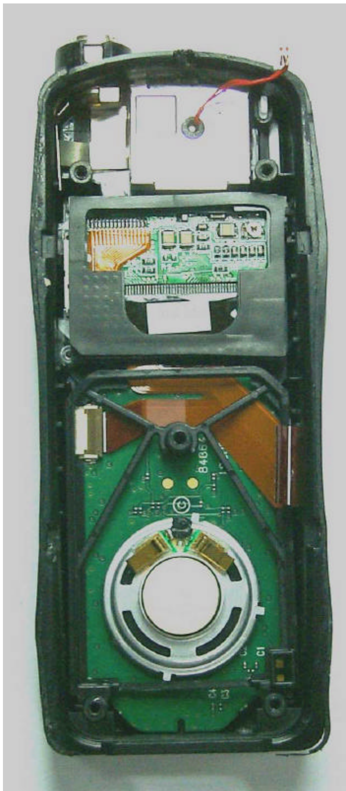
Photograph 9-3: Radio rear housing and main board removed, exploring inside of front housing, back side of display module and keypad with speaker.
