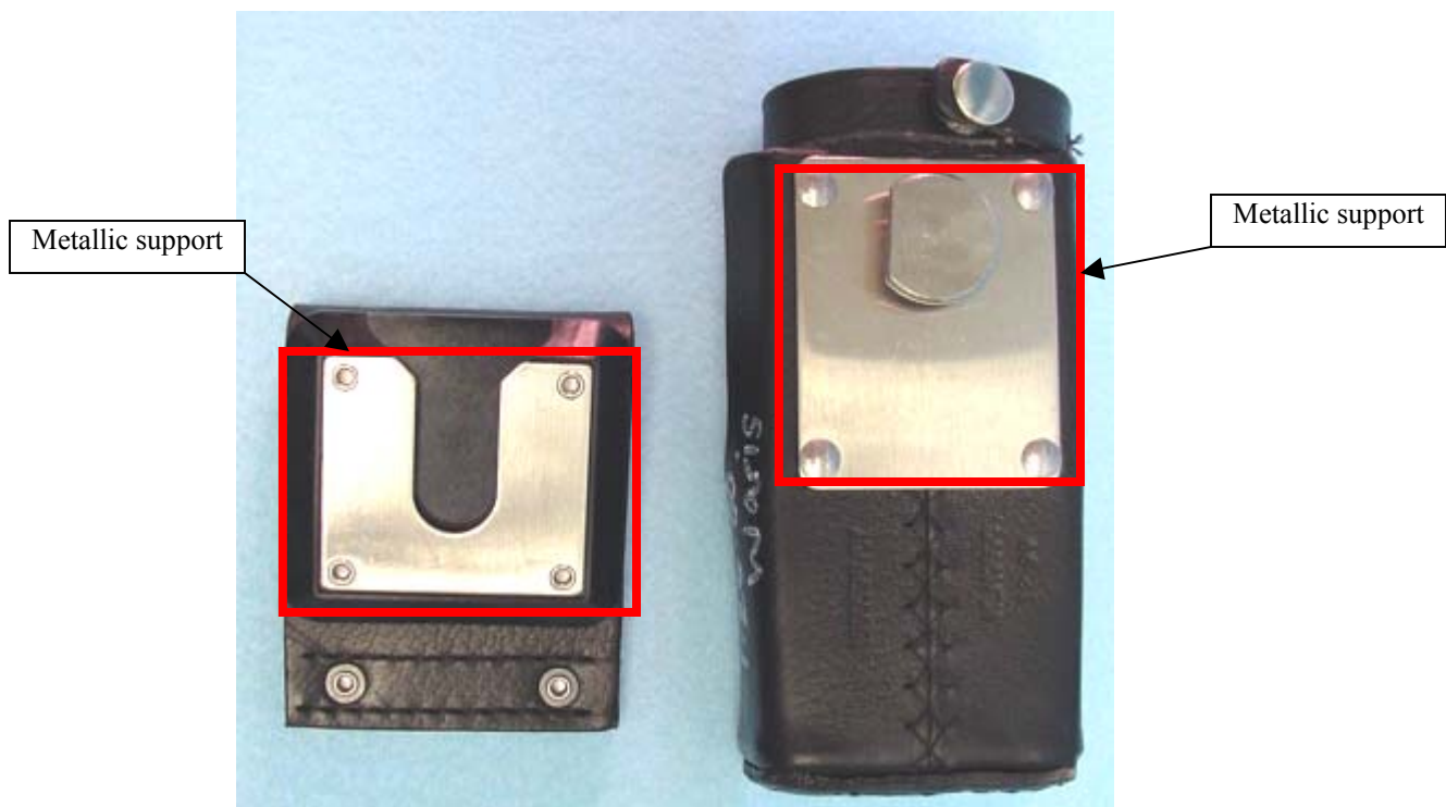
Photo 17, The HLN9690A has metallic supports for swivel purpose.
