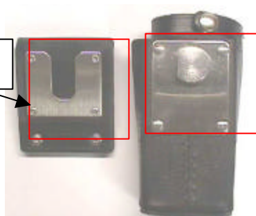
Photo 17, The HLN9690A has metallic supports for swivel purpose.
