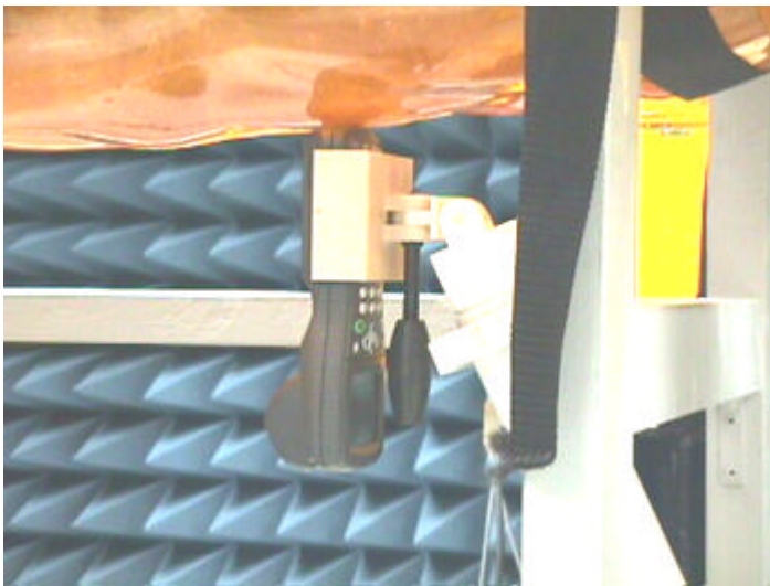
Figure 2: Bottom of Device perpendicular to the phantom. Distance from surface of device (bottom) to phantom = 0.0 mm
