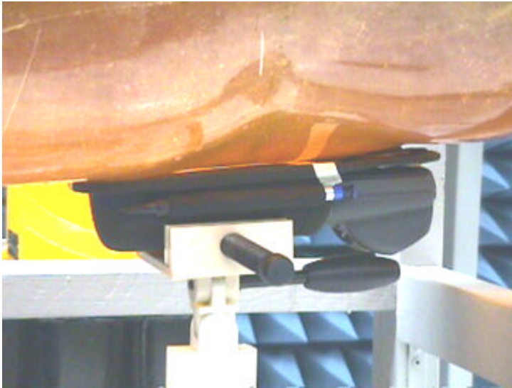
Figure 1: Hand-held data terminal (HDT502) and FLN9623A holster. Distance from the phantom to the HDT502 = 5.0 mm (Holster is 5.0 mm thick)
