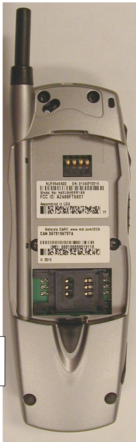
Photograph 3-5: Rear View of radio, battery removed to show FCC label location.
