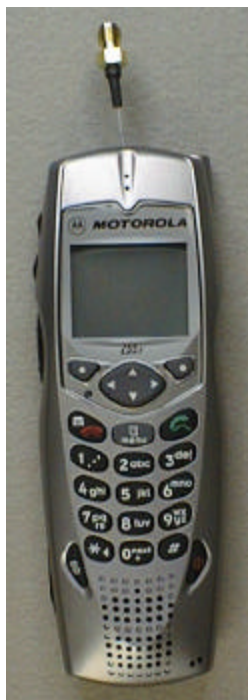
Photograph 7-1: Front view of radio with semi-rigid cable with female SMA connector soldered on the board.
