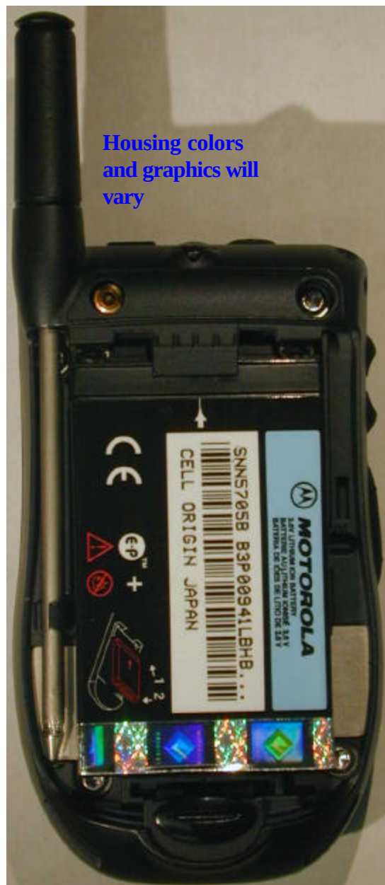
Photograph 3-4: Rear view of radio product, with standard battery (battery cover removed), antenna retracted and Motorola sticker removed.
