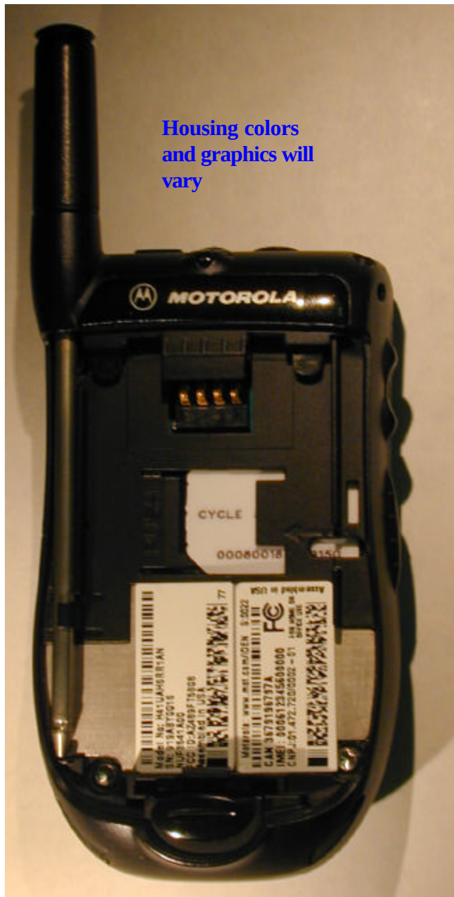
Photograph 3-5: Rear view of radio product, battery removed to show FCC and Industry Canada ID labels orientation.
