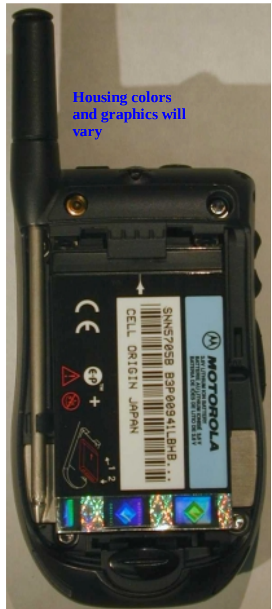
Photograph 3-4: Rear view of radio product, with standard battery (battery cover removed), antenna retracted and Motorola sticker removed.
