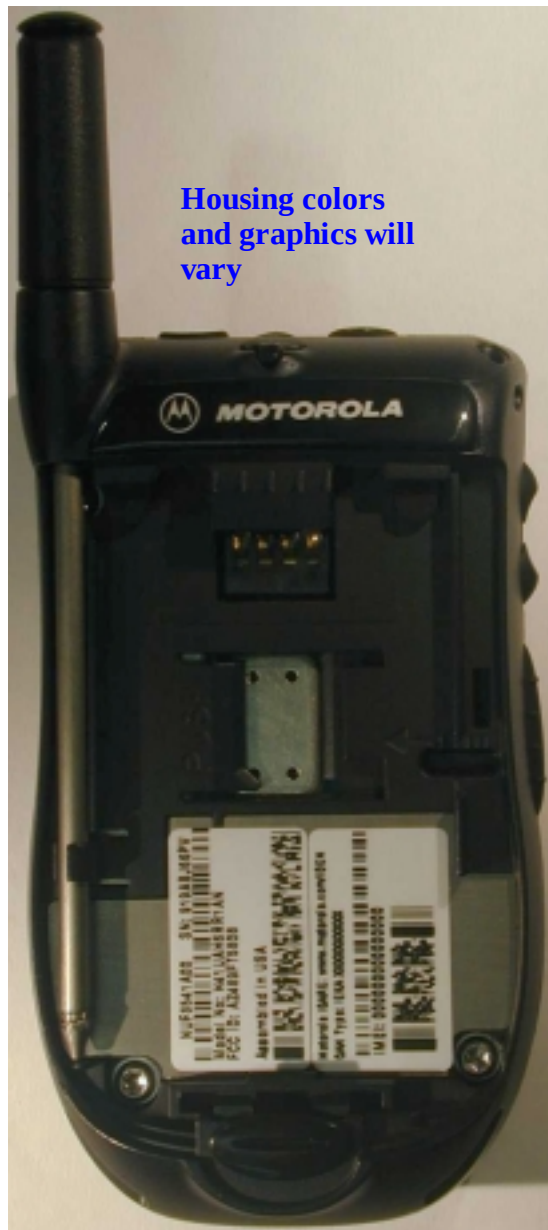
Photograph 3-5: Rear view of radio product, battery removed to show FCC and Industry Canada ID labels orientation.
