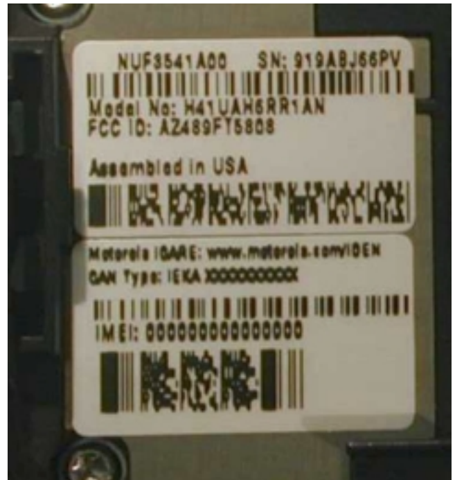
Photograph 3-6: Close up of the FCC and Industry Canada ID labels.
