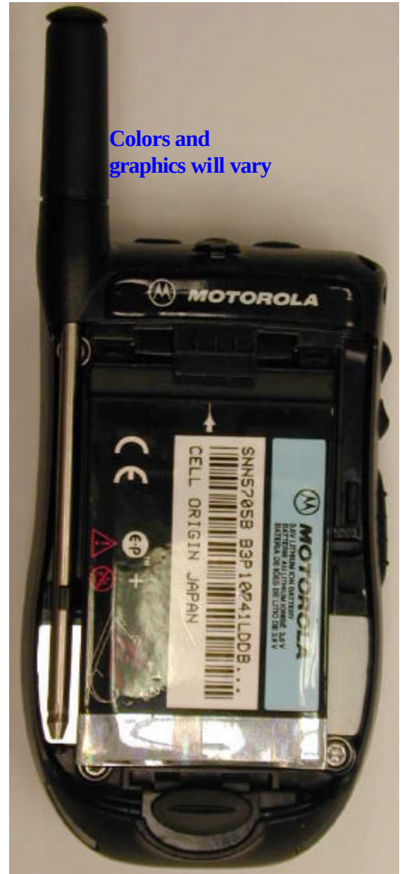
Photograph 3.2-4: Rear view of radio product, with standard battery (battery cover removed), antenna retracted.
