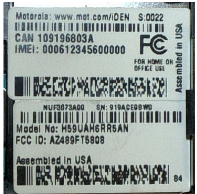
Photograph 3.2-6: Close up of the FCC and Industry Canada ID labels for the radio product.
