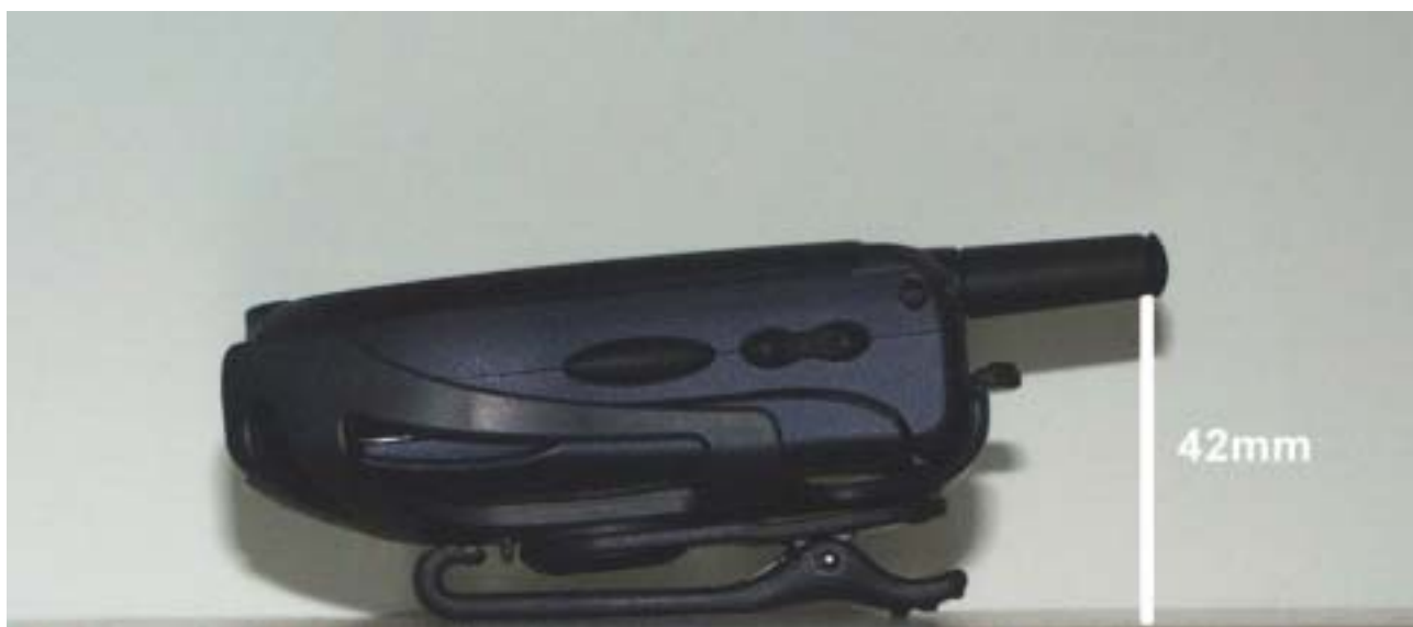
Figure 15. Separation Distance Provided by Belt Clip with Antenna Retracted
