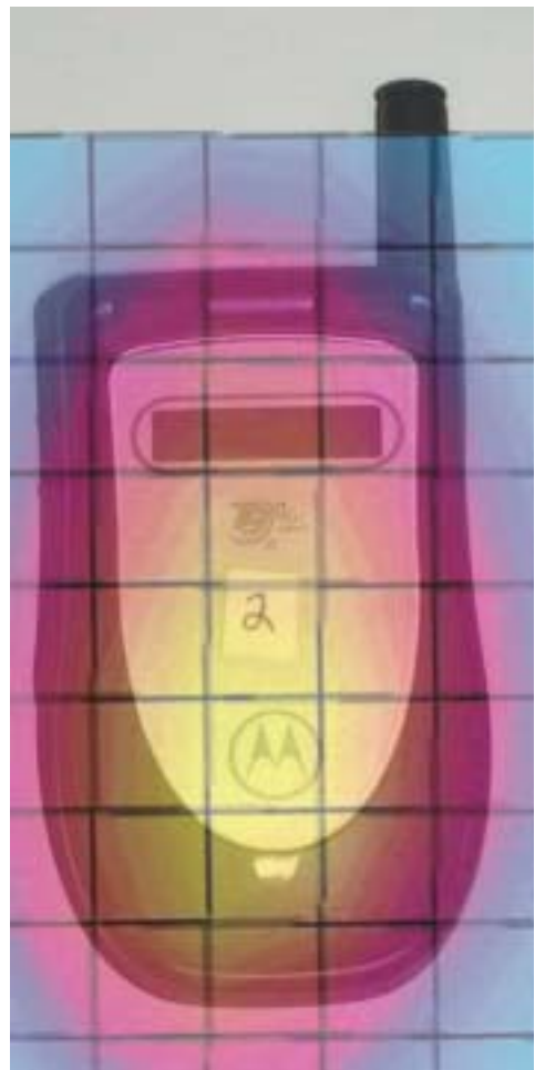
Figure 4. Typical Contour Plot for P-T-T Mode with Antenna Retracted Overlaid on Front of Radio
