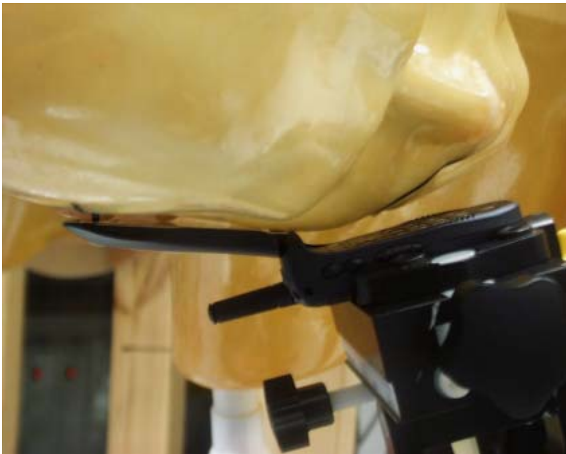
Figure 13. Radio with Antenna Retracted in Cheek Touch Position
