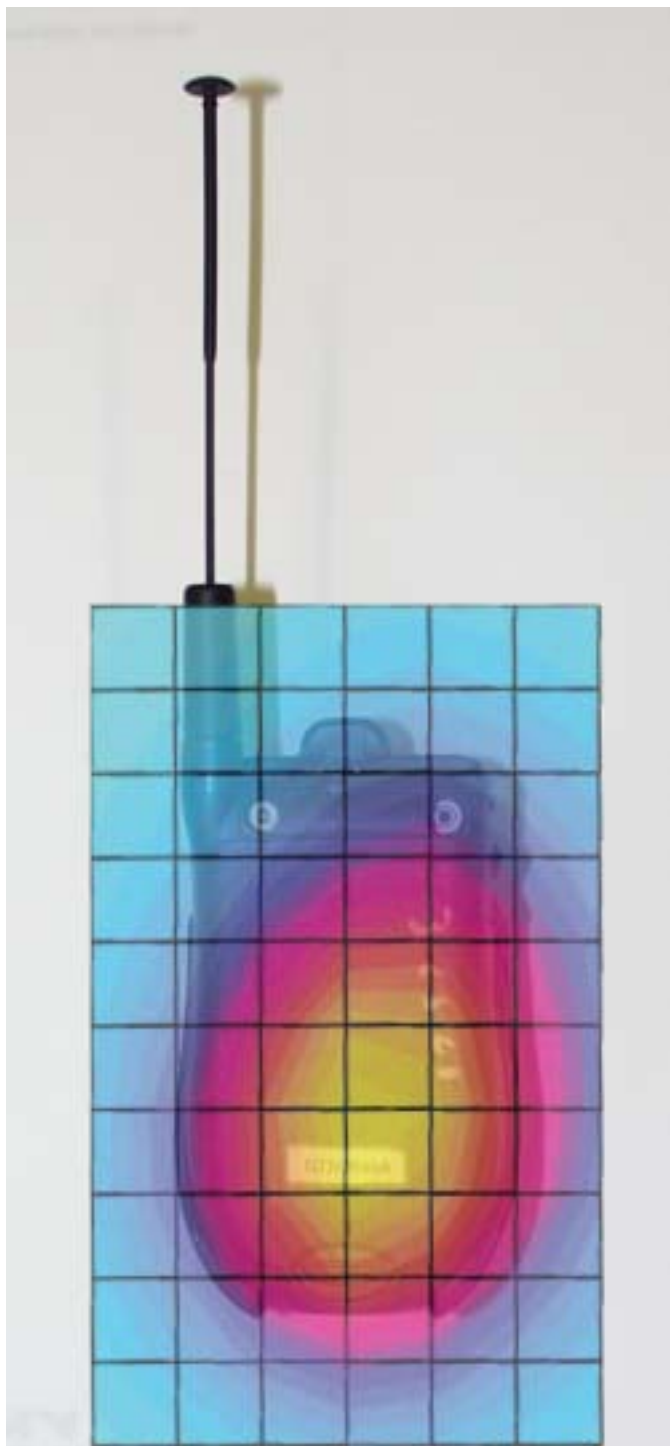
Figure 5. Typical Contour Plot for Data Mode with Antenna Extended Overlaid on Back of Radio
