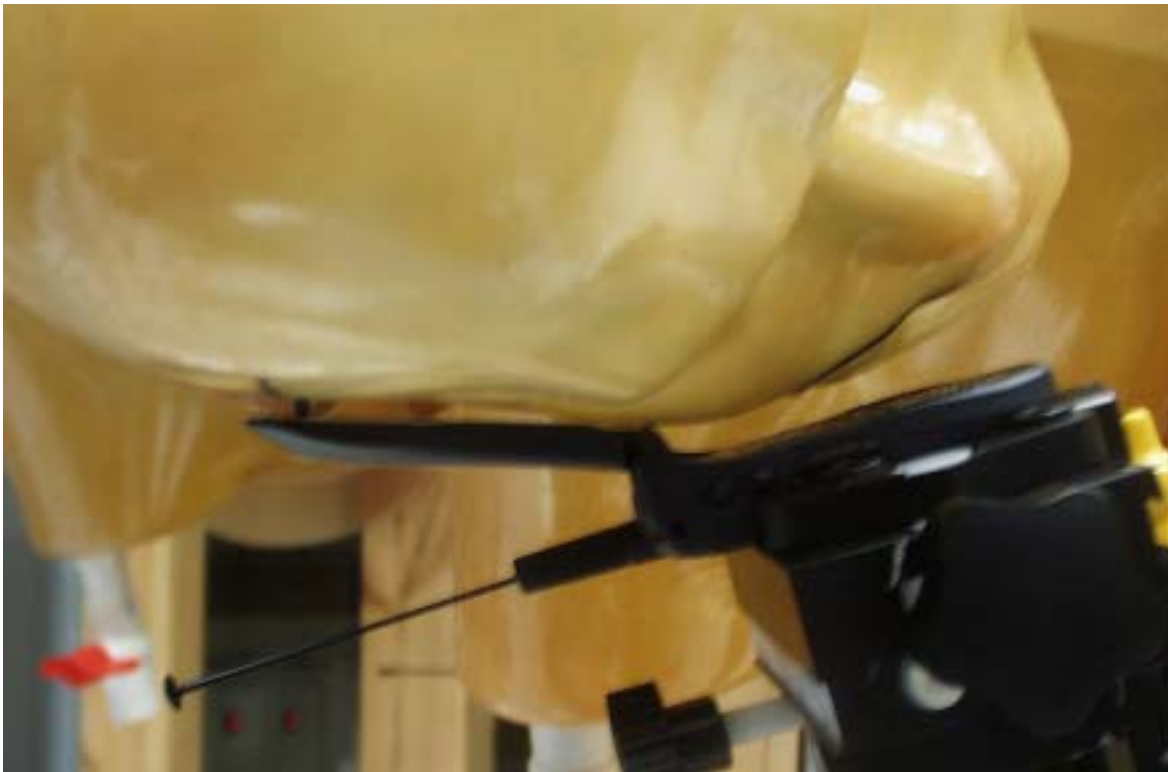
Figure 12. Radio with Antenna Extended in Cheek Touch Position
