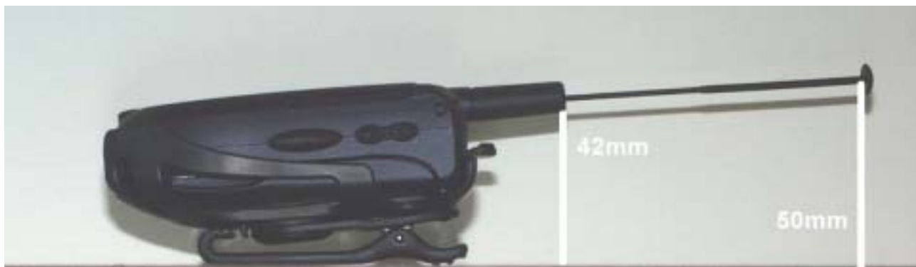
Figure 14. Separation Distance Provided by Belt Clip with Antenna Extended
