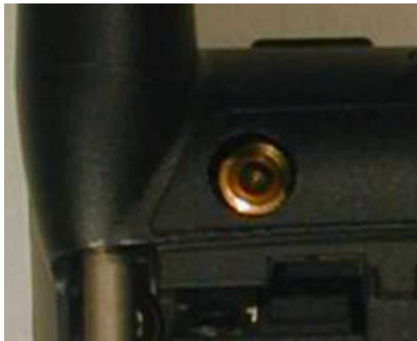
Photograph 7-1: i90c RF test switch.
