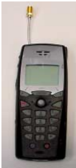
Photograph 7-1: Front view of radio with semi-rigid cable with female SMA connector soldered on the board.
