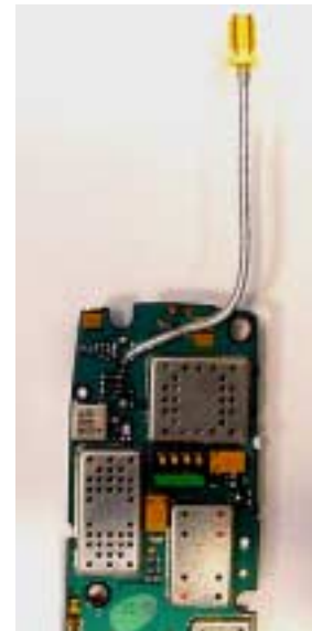
Photograph 7-2: Back side of main circuit board showing a semi-rigid cable with female SMA connector soldered on the board.
