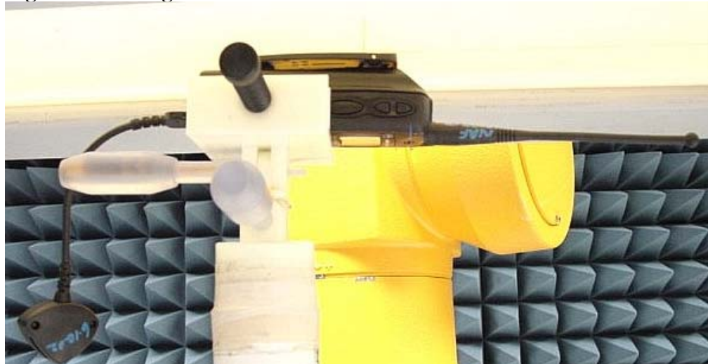
Figure 7. DUT against Flat Phantom w/ HLN9714A&NKN6503B attached
