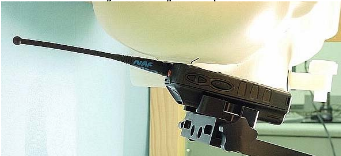
Figure 4. DUT Right ear Tilt position
