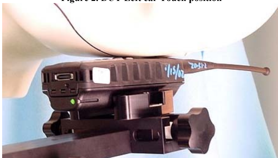
Figure 2. DUT Left ear Touch position
