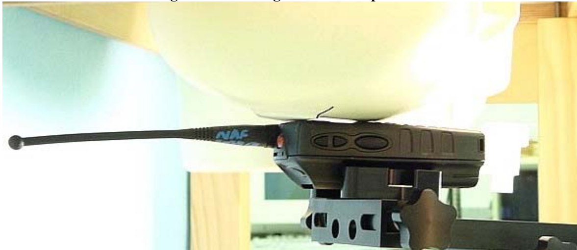
Figure 3. DUT Right ear Touch position
