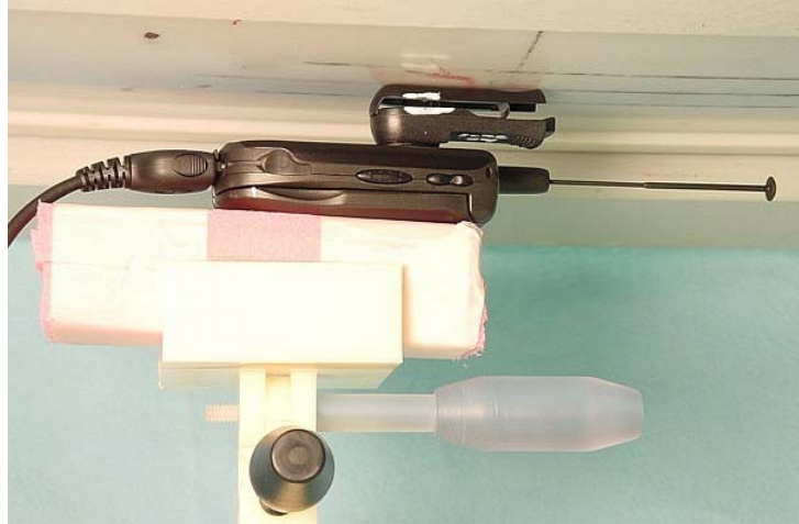
Figure 8. Assessment @ Body DUT w/ belt clip model NNTN4747A against the flat phantom (With offered data cable attached; same position used with offered audio accessories attached)
