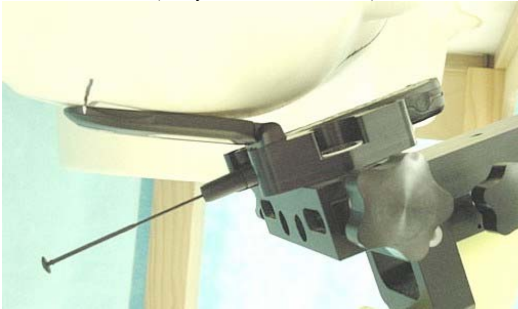
Figure 6. Assessment @ the Face (Flip opened) DUT front 2.5cm separation distance from flat phantom.
