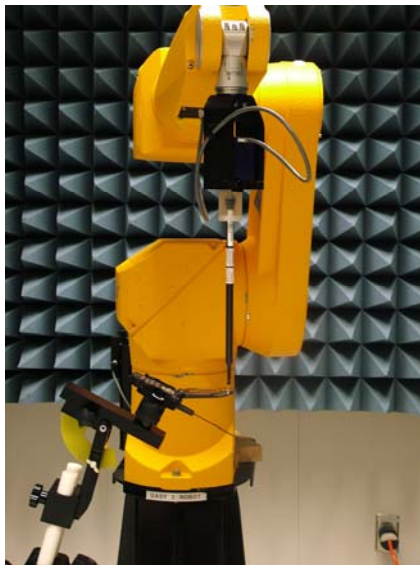
DUT test setup with 10mm spacing
