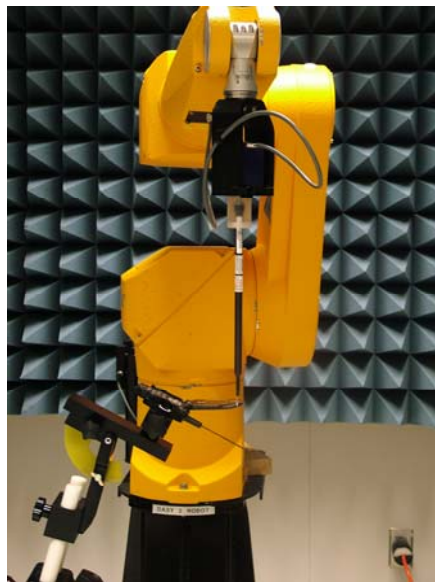
DUT test setup with 10mm spacing
