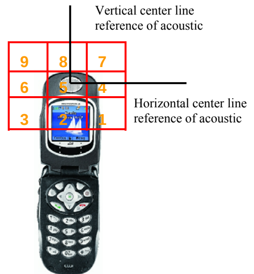
Example illustration of WD with reference grid (Not to scale)
