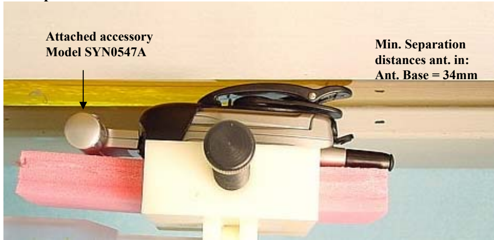
Figure 9. Assessment @ the Abdomen; with carry case model NNTN4682A against the phantom and attached digital camera model SYN0547A. Same position used for antenna extended
