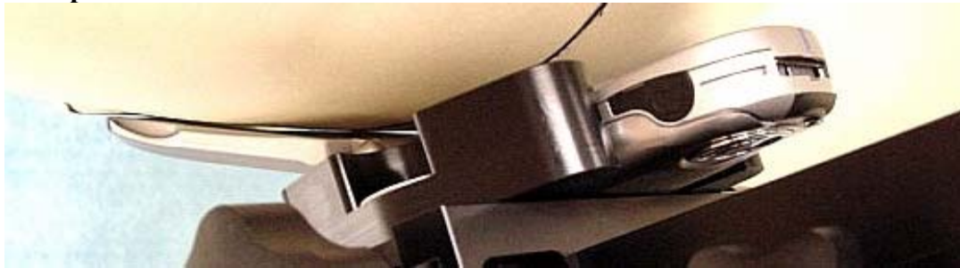
Figure 4. Assessment @ the Right ear; Cheek touch position; with antenna retracted. Same position used for antenna extended.
