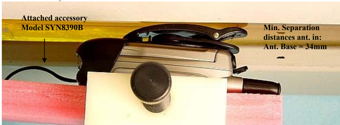
Figure 10. Assessment @ the Abdomen; with carry case model NNTN4682A against the phantom and attached audio accessory model SYN8390B. Same position used to assess audio accessory models SYN8146C, NTN8513B, SYSN7875C, NTN8496A, NNTN4033A, and NSN6066A w/ antenna in and out.
