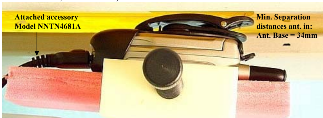
Figure 8. Assessment @ abdomen; DUT w/ carry case model NNTN4682A against the flat phantom and attached data cable model NKN6544B. Same position used to assess data cable models NKN6540A, NNTN4007A, NNTN4049A, NNTN4877A, and SYN0547A w/ antenna in and out.
