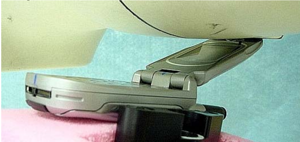
Figure 3. Assessment @ the Left ear; 15° tilt position; with antenna retracted. Same position used for antenna extended.
