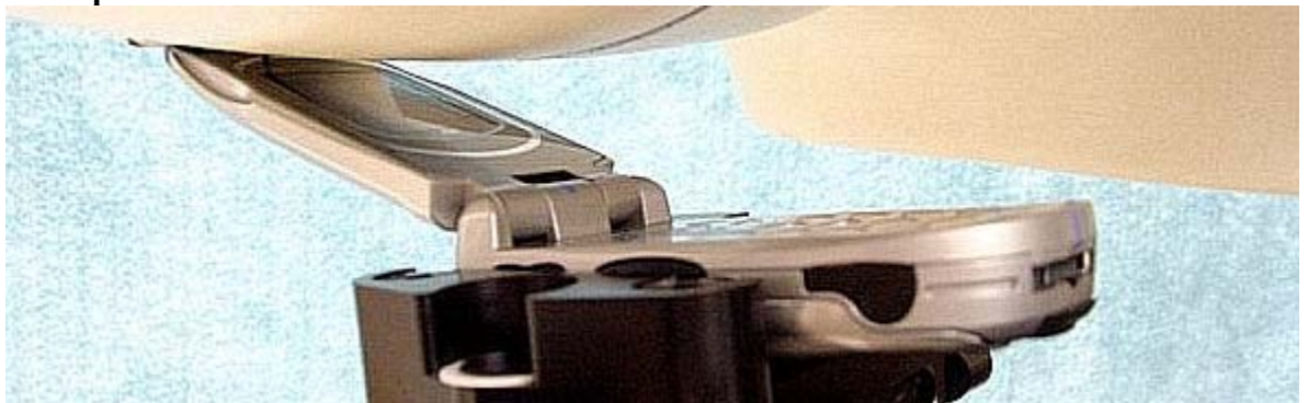
Figure 5. Assessment @ the Right ear; 15° tilt position; with antenna retracted. Same position used for antenna extended.
