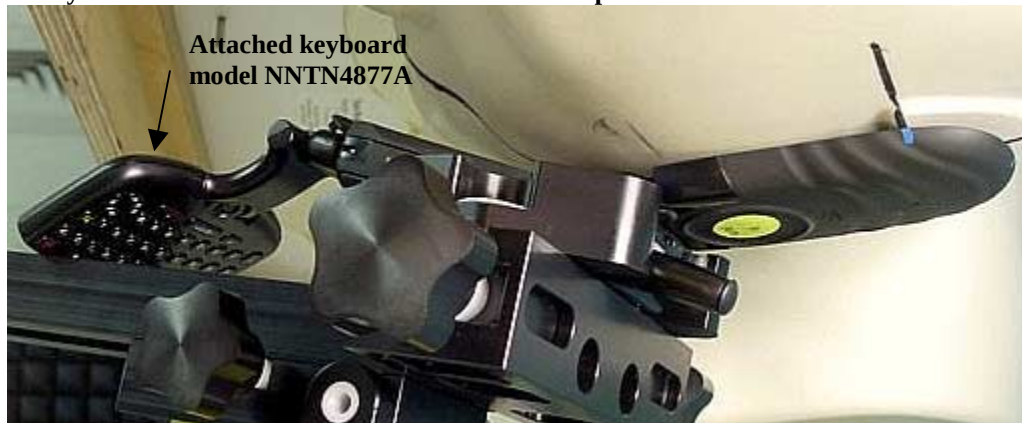
Figure 6. Assessment @ the Left ear; cheek touch position; w/ keyboard attached and antenna retracted. Same position used for antenna extended.
