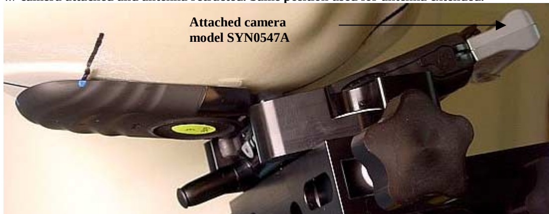
Figure 7. Assessment @ the Right ear; cheek touch position; w/ camera attached and antenna retracted. Same position used for antenna extended.
