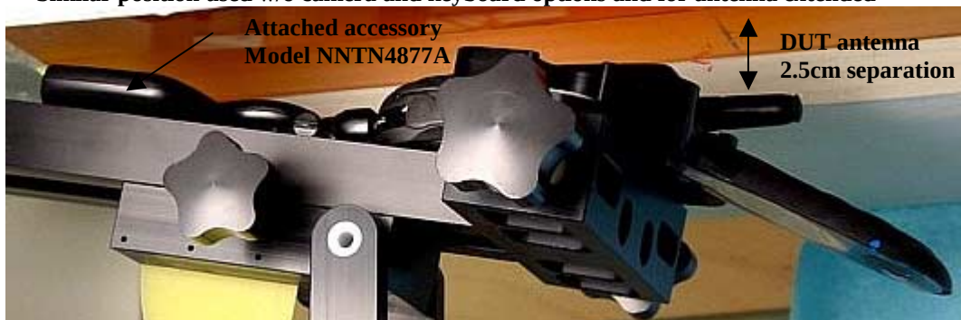
Figure 15. Assessment @ the Abdomen; DUT back towards phantom w/ attached keyboard and antenna separated 2.5cm. Similar position used w/o camera and keyboard options and for antenna extended
