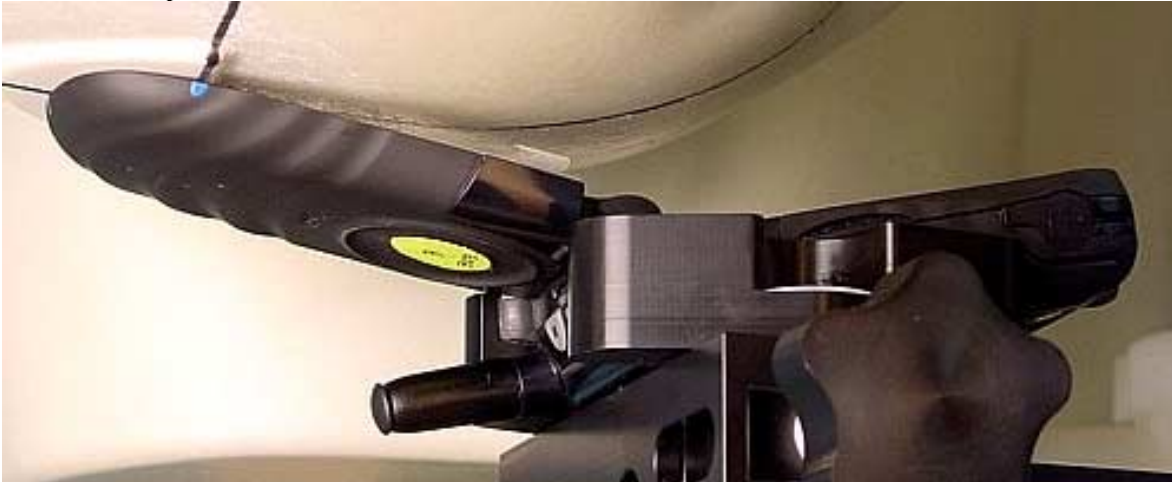
Figure 4. Assessment @ the Right ear; 15° tilt position; with antenna retracted. Same position used for antenna extended.
