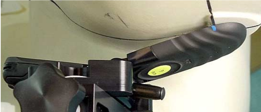
Figure 3. Assessment @ the Left ear; 15° tilt position; with antenna retracted. Same position used for antenna extended.
