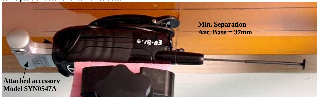
Figure 12. Assessment @ the Abdomen; w/holster model NNTN4756A against the phantom and attached digital camera model SYN0547A. Same position used for antenna retracted
