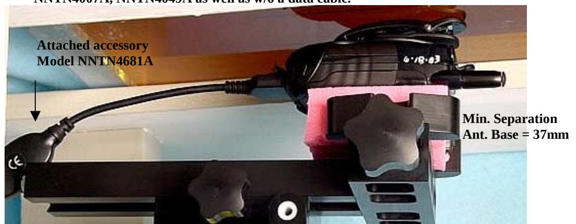
Figure 11. Assessment @ abdomen; DUT w/holster model NNTN4756A against the flat phantom and attached data cable model NKN6544B. Same position used for antenna extended and to assess data cable models NKN6540A, NNTN4007A, NNTN4049A as well as w/o a data cable.
