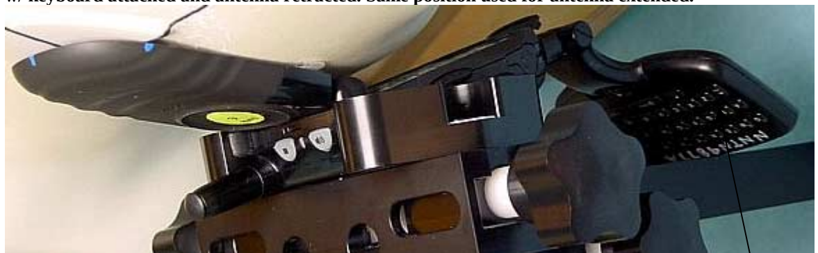
Figure 8. Assessment @ the Right ear; cheek touch position; w/ keyboard attached and antenna retracted. Same position used for antenna extended.
