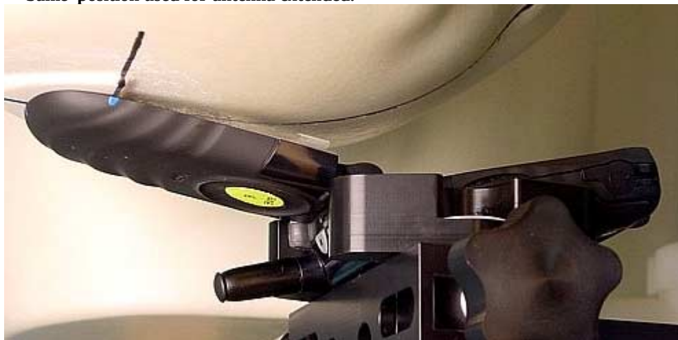
Figure 2. Assessment @ the Left ear; Cheek touch position; with antenna retracted. Same position used for antenna extended.
