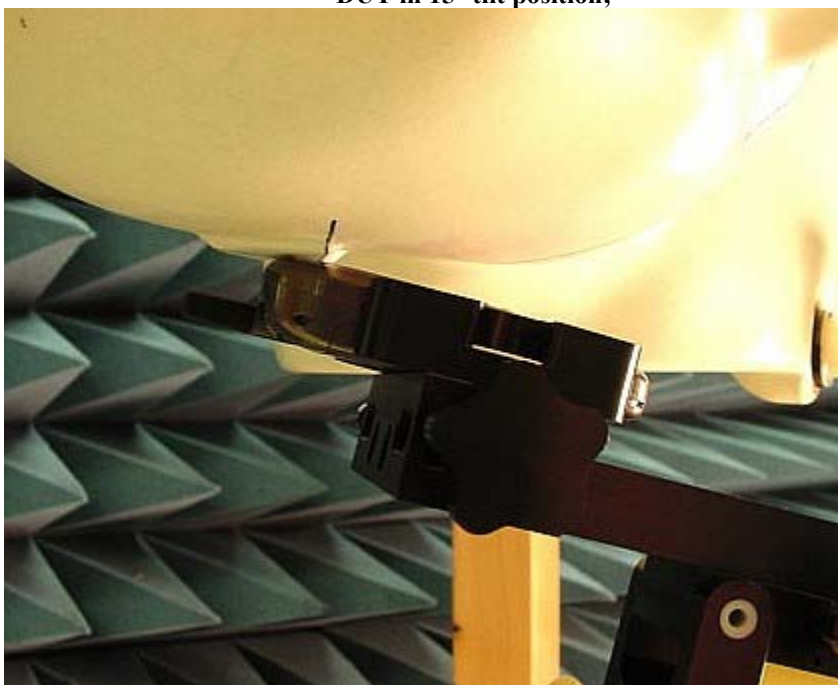
Figure 4. Assessment @ the Right ear DUT in 15° tilt position;
