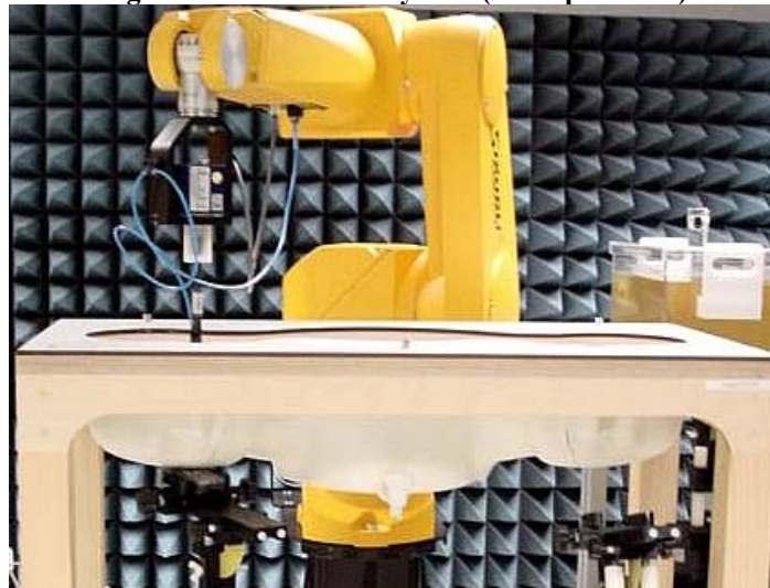
Figure 11: Robot Test System (SAM phantom)
