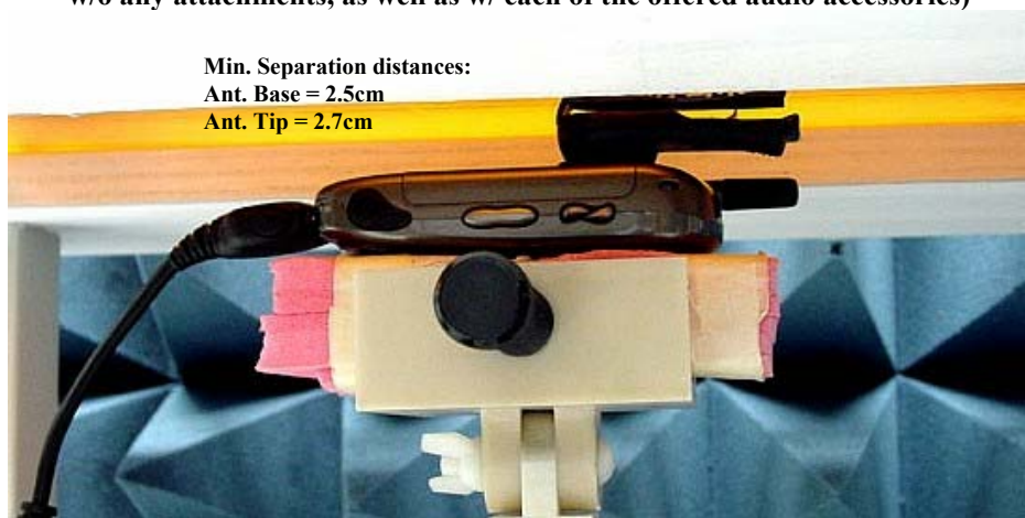
Figure 7. Assessment @ the Body DUT w/ belt clip model NNTN4747A and attached data cable model NKN6560A. (Same position used w/ data cable model NKN6559A attached, w/o any attachments, as well as w/ each of the offered audio accessories)
