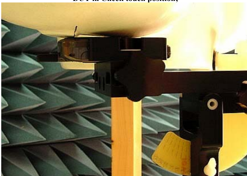
Figure 3. Assessment @ the Right ear DUT in Cheek touch position;
