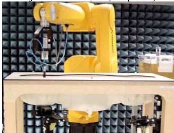
Figure 11: Robot Test System (SAM phantom)
