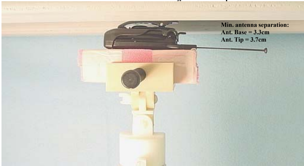
Figure 8. Assessment @ Body DUT w/ belt clip model NNTN4747A against the flat phantom With data cable model NKN6 559A attached; (same position used with other data cable as well as with offered audio accessories attached)
