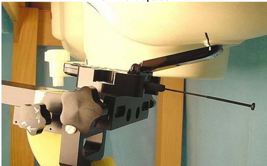
Figure 3. Assessment @ the Left ear DUT in Cheek touch position
