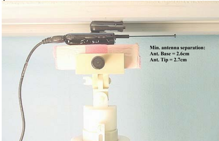
Figure 8. Assessment @ Body DUT w/ belt clip model NNTN4747A against the flat phantom With data cable model NKN6 559A attached; (same position used with other data cable as well as with offered audio accessories attached)
