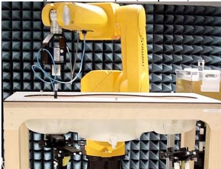
Figure 11: Robot Test System (SAM phantom)
