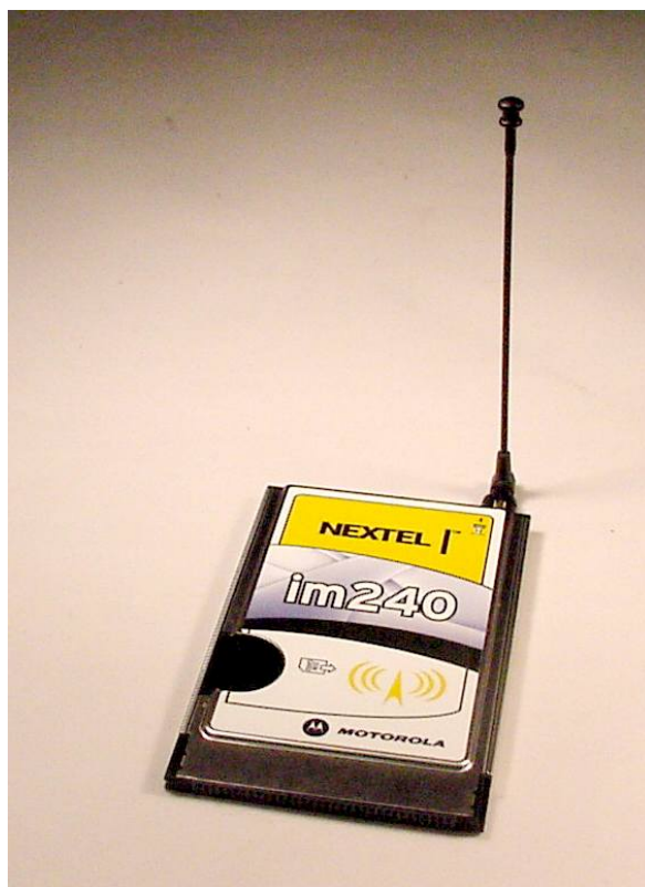
Figure 3-2. Photograph of Front, antenna installed.
