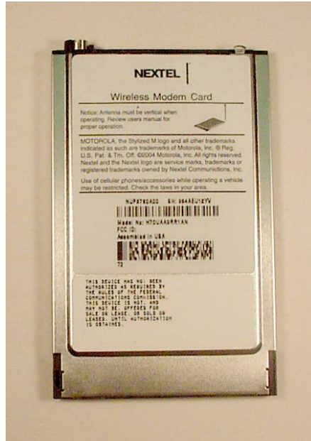
Figure 3-3. Photograph of back showing location of FCC label.
