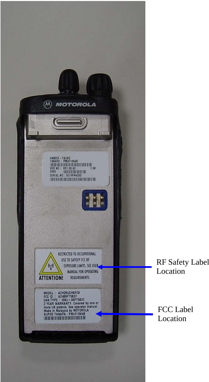
Figure 3-6: Rear view of complete radio showing FCC Label
