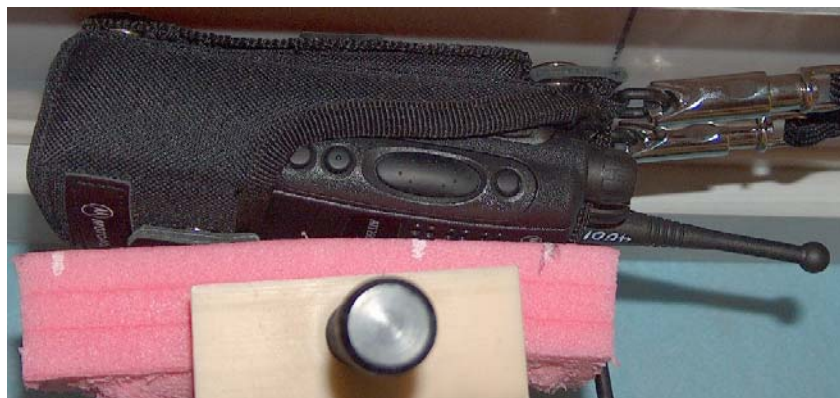
Figure 10: Test Position (Body); Antenna model PMAF4001A DUT w/carry case model HLN9701B w/carry strap NTN5243A against the phantom; audio acc. model HMN9030A w/HLN9716C attached
