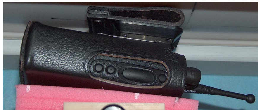
Figure 7: Test Position (Body); Antenna model PMAF4001A DUT w/carry case model HLN9670A w/NTN8039B against the phantom; audio acc. model HMN9030A w/HLN9716C attached
