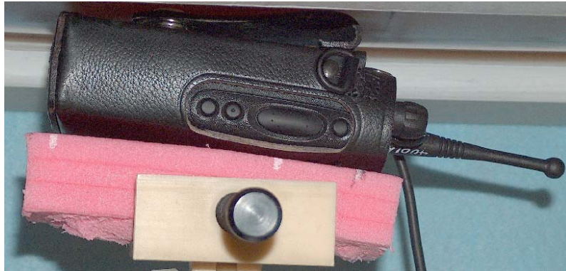
Figure 5: Test Position (Body); Antenna model PMAF4001A DUT w/carry case model HLN9652A against the phantom; audio acc. model HMN9030A w/HLN9716C attached
