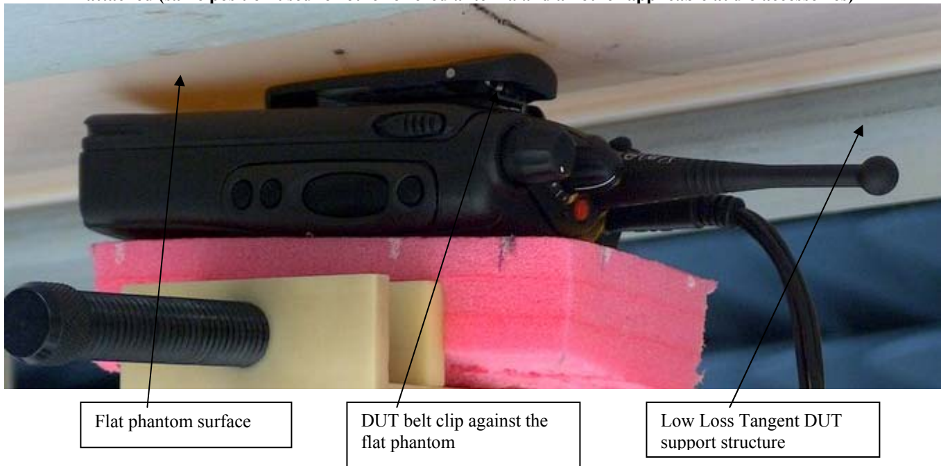
Figure 1: Highest S.A.R. Test Position (Body); Antenna model PMAF4001A DUT w/belt clip model HLN9844A against the phantom; worst case audio acc. model BDN6730A w/HLN9717A attached (same position used for other offered antenna and all other applicable audio accessories)
