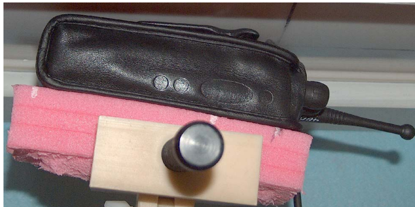
Figure 15: Test Position (Body); Antenna model PMAF4001A DUT w/carry case model PMLN4280A against the phantom; audio acc. model HMN9030A w/HLN9716C attached
