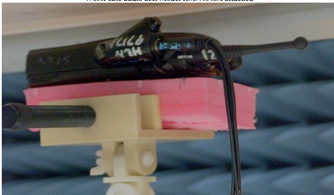
Figure 4: Body Assessment DUT w/ front housing separated 2.5cm from the phantom Worst case audio acc. Model RMN4048A attached
