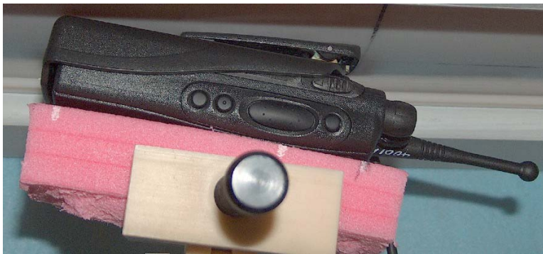
Figure 12: Test Position (Body); Antenna model PMAF4001A DUT w/carry case model HLN9952A and belt clip model HLN9844A against the phantom; audio acc. model HMN9030A w/HLN9716C attached
