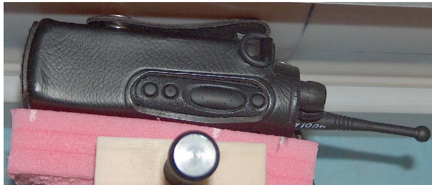
Figure 6: Test Position (Body); Antenna model PMAF4001A DUT w/carry case model HLN9655A against the phantom; audio acc. model HMN9030A w/HLN9716C attached
