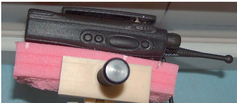
Figure 13: Test Position (Body); Antenna model PMAF4001A DUT w/belt clip model HLN9714A against the phantom; audio acc. model HMN9030A w/HLN9716C attached
