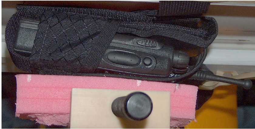
Figure 14: Test Position (Body); Antenna model PMAF4001A DUT w/fanny pack model RLN4815A against the phantom; audio acc. model HMN9030A w/HLN9716C attached
