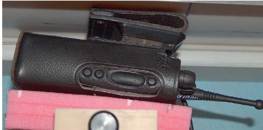
Figure 8: Test Position (Body); Antenna model PMAF4001A DUT w/carry case model HLN9676A w/NTN8039B against the phantom; audio acc. model HMN9030A w/HLN9716C attached
