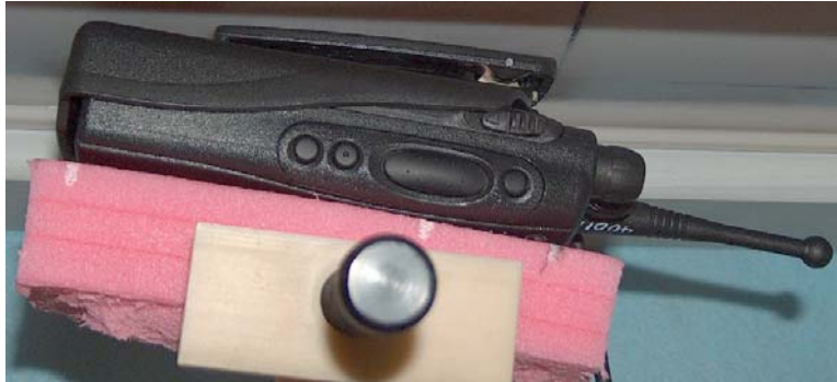
Figure 11: Test Position (Body); Antenna model PMAF4001A DUT w/carry case model HLN9952A and belt clip model HLN9714A against the phantom; audio acc. model HMN9030A w/HLN9716C attached
