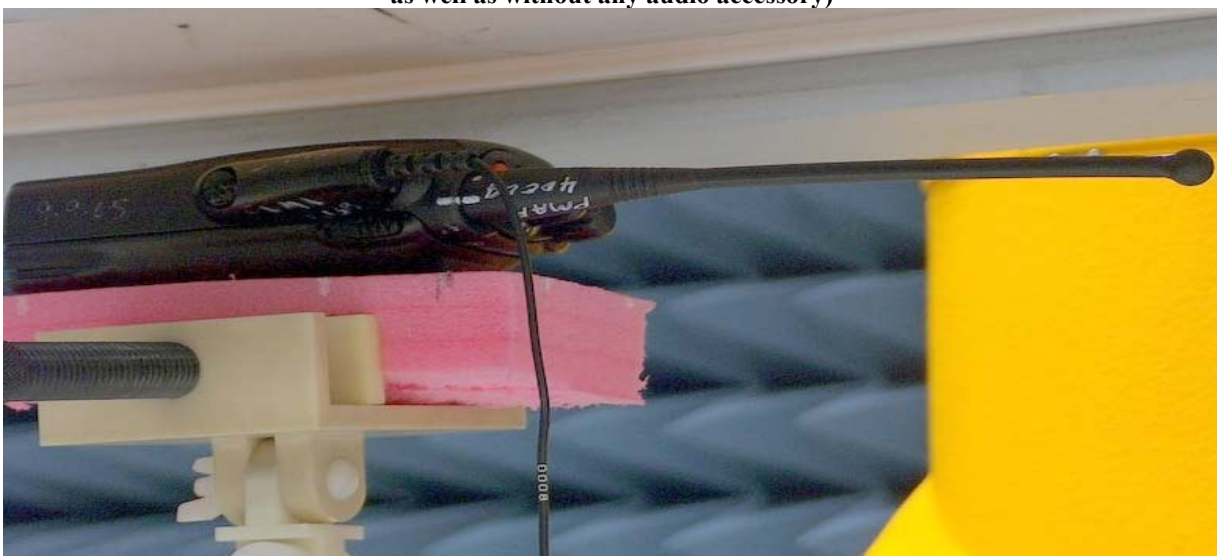
Figure 2: Highest S.A.R. Test Position (face); Antenna model PMAF4000A DUT front side separated 2.5cm from the phantom; w/audio accessory Model ENMN4013A attached (same position used for other offered antenna, all other applicable audio accessories, as well as without any audio accessory)
