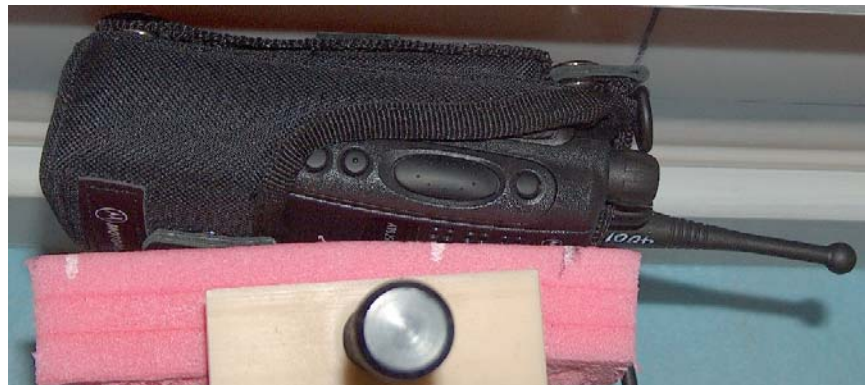
Figure 9: Test Position (Body); Antenna model PMAF4001A DUT w/carry case model HLN9701B against the phantom; audio acc. model HMN9030A w/HLN9716C attached
